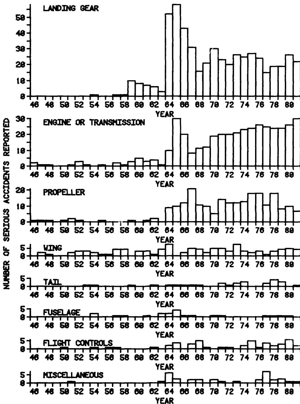
FIG. 4 CAUSES OF FATIGUE FAILURES - FIXED-WING AIRCRAFT
