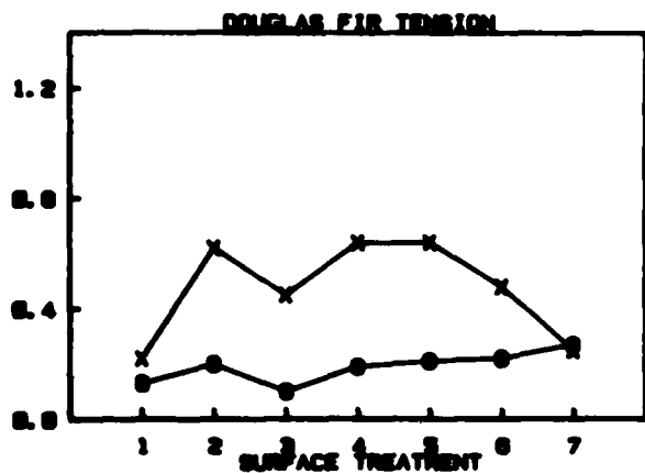
Figure 19.--Coefficients of variation of the six abrasive planing treatments and one knife planing treatment average strengths (Douglas-fir tension). Surface treatments 1-6 are abrasive, treatment 7 is knife planed. Treatments 1-6 are as follows: (1) 45 fpm/0.010-inch cut, (2) 45/0.040, (3) 45/0.080, (4) 90/0.010, (5) 90/0.040, (6) 90/0.080.
