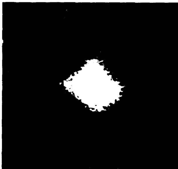
Figure 31. Far-field pattern taken at 47.8 kV discharge (Shot number 7210) 7X enlargement.
