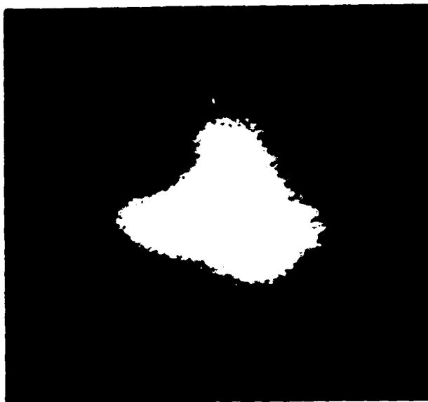
Figure 32. Far-field pattern taken at 47.8 kV discharge (Shot number 7208) 7X enlargement.
