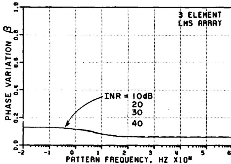
Figure 18. Phase Variation vs. Pattern Frequency
