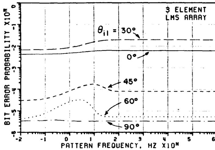
Figure 15. Bit Error Probability vs. Pattern Frequency
