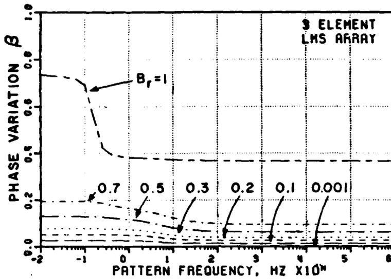
Figure 8. Phase Variation vs. Pattern Frequency
