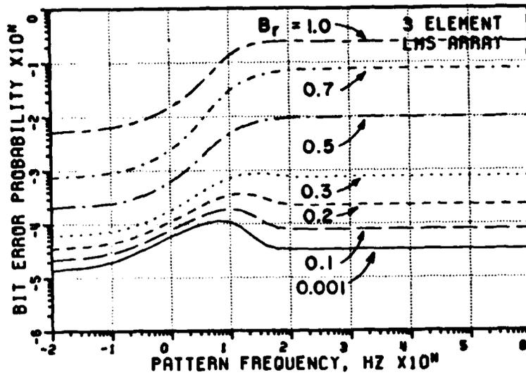
Figure 10. Bit Error Probability vs. Pattern Frequency
