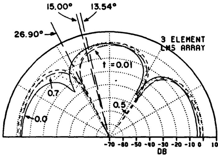
Figure 3. Array Patterns During Hopping Period
