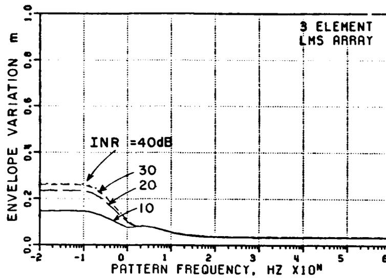
Figure 16. Envelope Variation vs. Pattern Frequency
