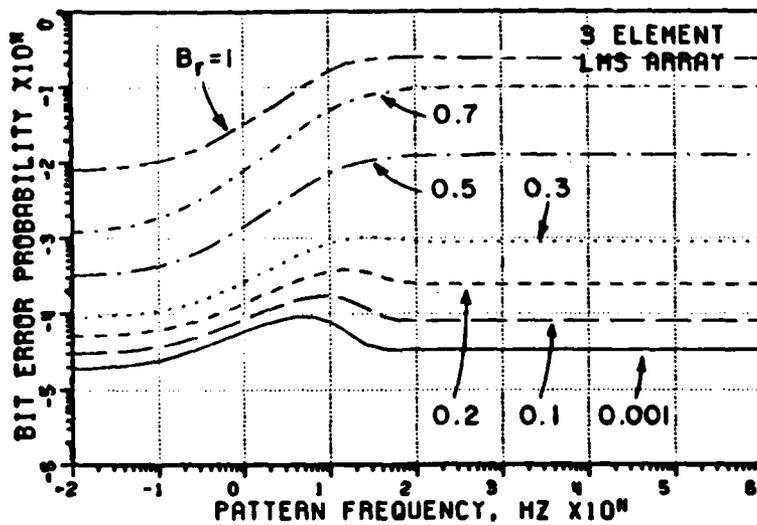
Figure 9. Bit Error Probability vs. Pattern Frequency
