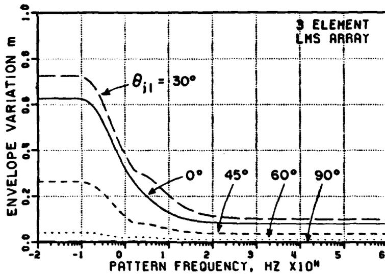
Figure 12. Envelope Variation vs. Pattern Frequency
