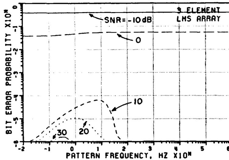
Figure 19. Bit Error Probability vs. Pattern Frequency
