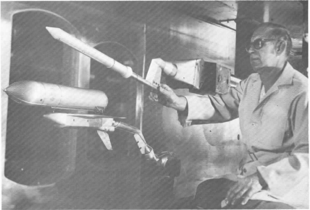
Figure 7. Test installation of a single-booster Space Shuttle staging test in Tunnel A.
