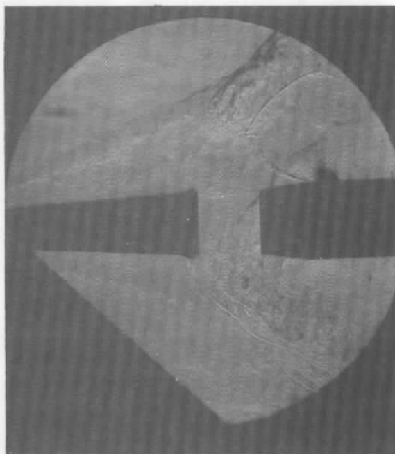
Figure 10. Schlieren photograph showing stage venting interference during in-line staging maneuver.
