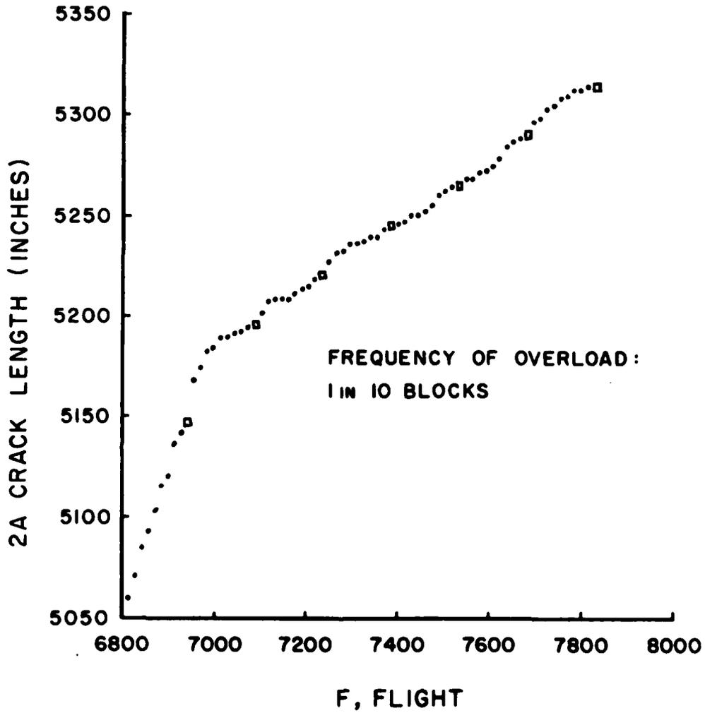
Figure 7. Constant K Crack Growth Affected by Overloads of One in Ten Blocks
