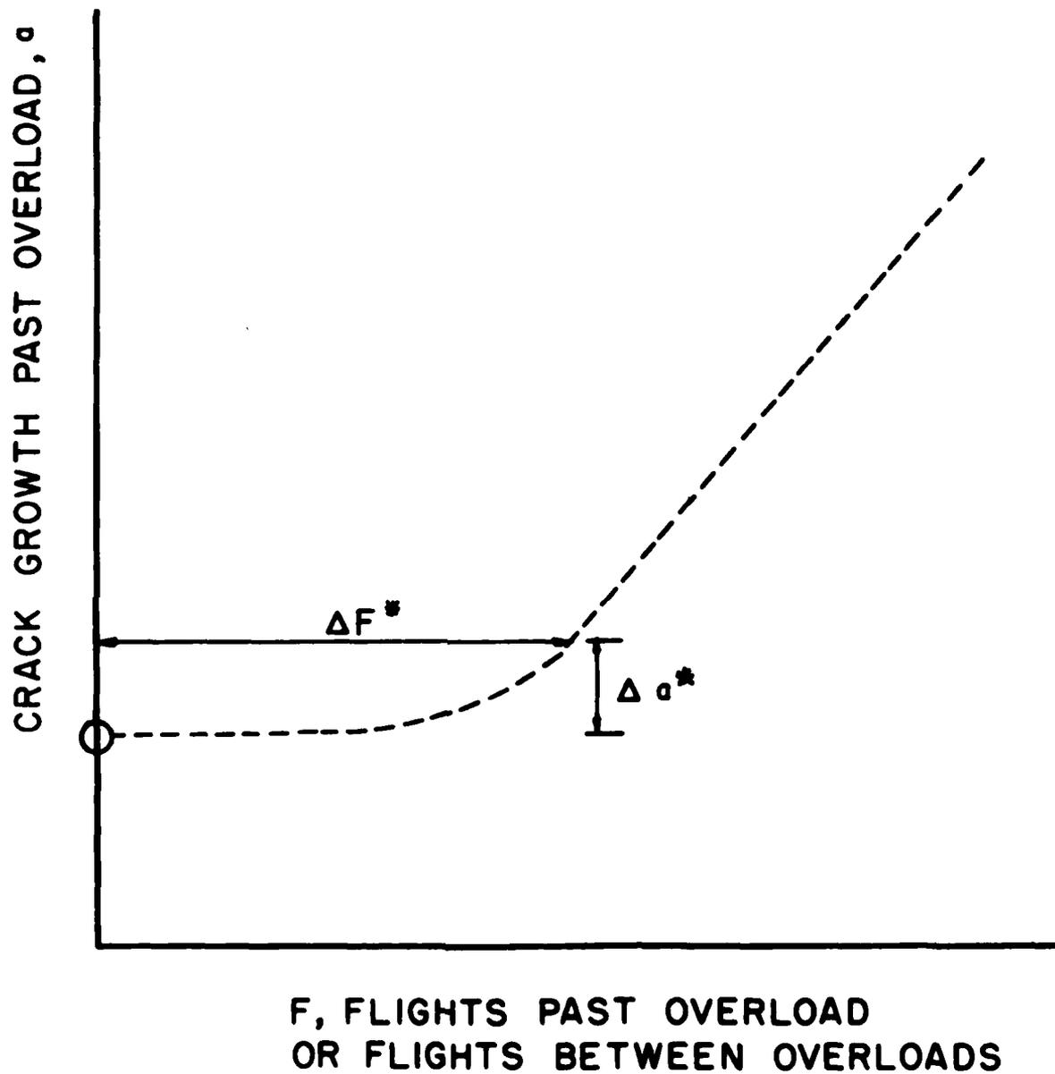
Figure 1. Schematic of Crack Length versus Flights Past Overload
