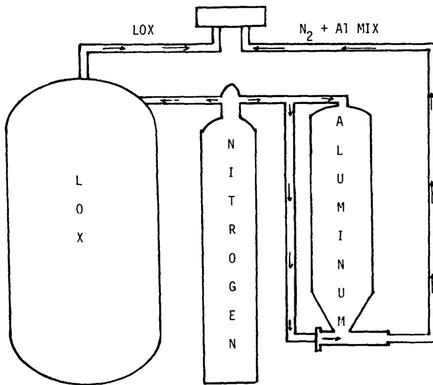
FIGURE 1. LOX TRS SCHEMATIC.
