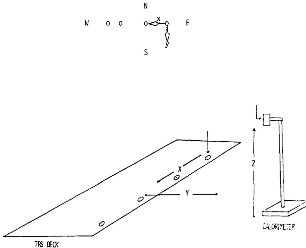
Figure A-1. Flux Gauge Co-ordinate System.
