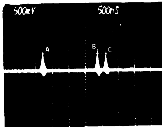
Figure 4.10: Echoes from different planes of the steel bond.
