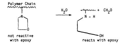
Upon exposure to water, the oxazolidine ring (which will not react with an epoxy prepolymer) will open to give a hydroxyl and amine group both of which will react with and crosslink the epoxy prepolymer. The water is provided by moisture in the air or on the bilge walls (i.e., after surface preparation by detergent washing). These resins can be made with low vapor pressure aldehydes that will reduce or eliminate any emissions from the paint during drying.
