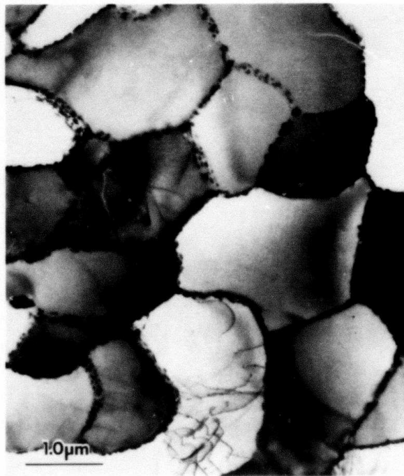
FIGURE 8. As spun ribbon of Al-12 wt.% Mn alloy. A cellular microstructure with particles at the cell boundaries is observed.
