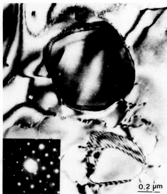
FIGURE 2. G phase particles. The diffraction pattern represents a [001] zone axis.
