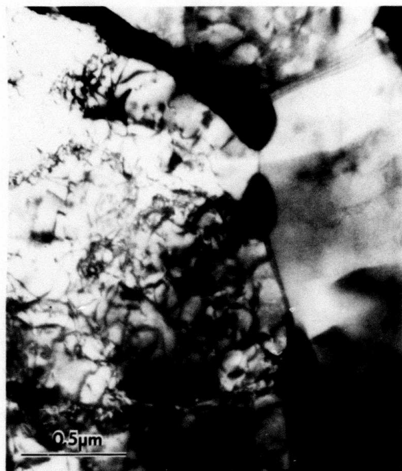
FIGURE 11. Al 3 Mn particles at cell boundary of Al-3 wt.% Mn alloy annealed 1 hour at 450°C.
