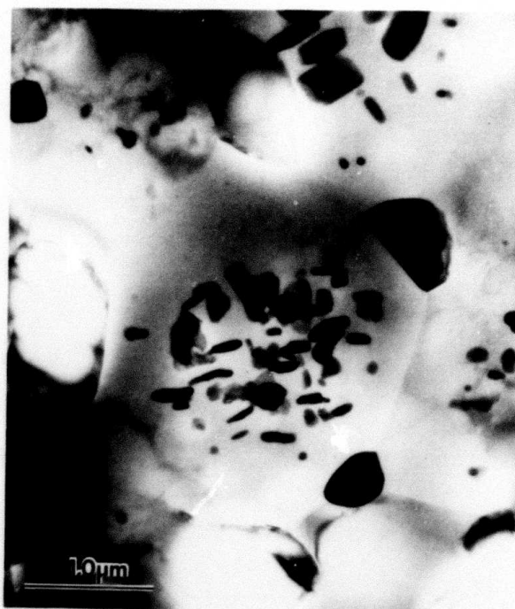
FIGURE 16. Al-5 wt.% Mn alloy following annealing for 65 hours at 450°C. T phase particles are found only in the center of the subgrains, and the depleted zone has grown.
