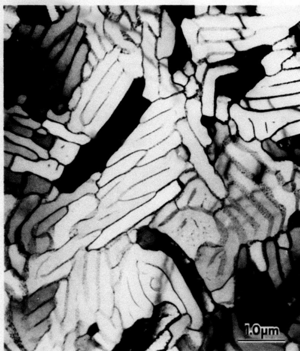
FIGURE 9. As spun ribbon of Al-15 wt.% Mn alloy. Note the contrast difference between cells indicating that the cells are also subgrains.
