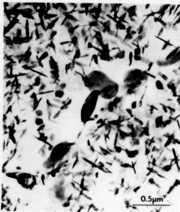
FIGURE 17. The microstructure of the Al-9 wt.% Mn alloy following 5 min. at 450°C.
