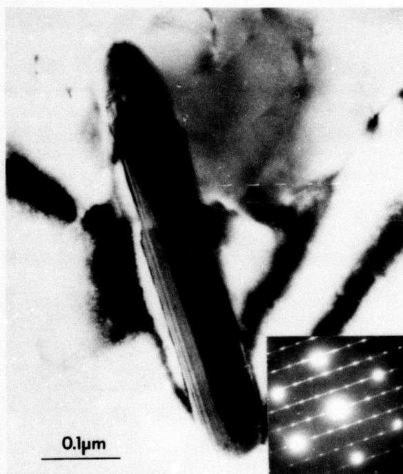
FIGURE 3. G'' phase particle. The diffraction pattern represents a [110] Aluminum zone axis and (2110) G'' zone axis.
