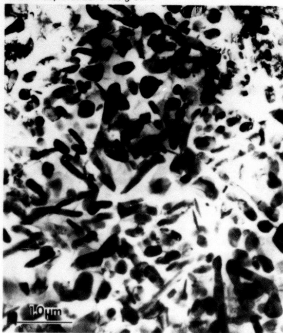
FIGURE 18. Al 6 Mn particles in the Al-9 wt.% Mn following 1 hour at 450°C.
