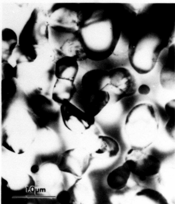
FIGURE 23a. Al 6 Mn particles in aluminum matrix. The microstructure of Al-15 wt.% Mn following 6 hours at 450°C.
