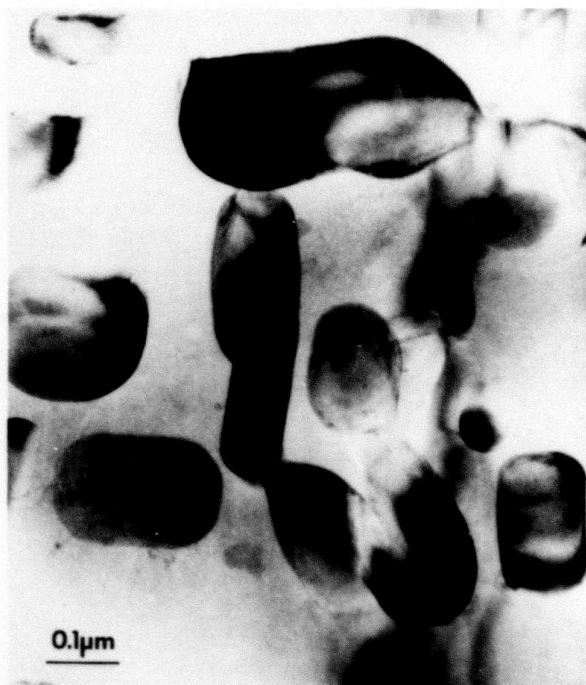
FIGURE 21. Coarse Al 6 Mn particles in Al-12 wt.% Mn following 1 hour at 450°C.
