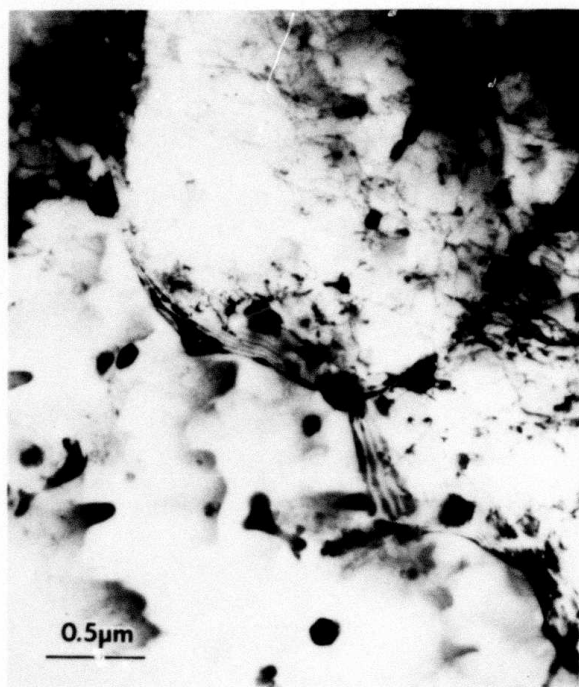
FIGURE 6. As spun thick ribbon of Al-5 wt.% alloy. Particles are seen at cell boundaries.
