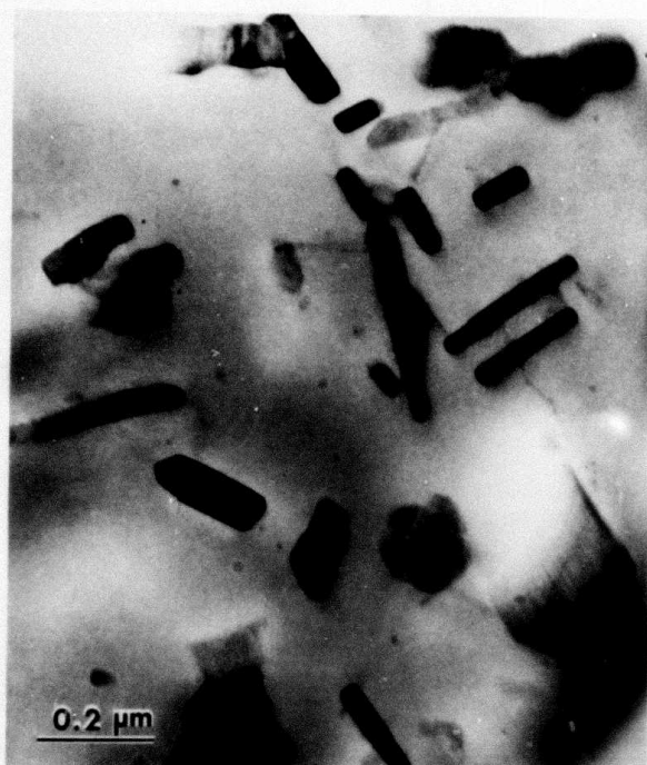
FIGURE 15. Coarsening of the T phase in Al-5 wt.% Mn annealed for 16 hours at 450°C.
