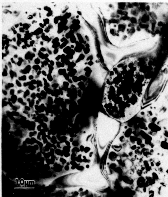
FIGURE 19. The Al-9 wt.% Mn alloy following 16 hours at 450°C containing Al 6 Mn particles within the grains and almost continuous G phase at subgrain boundaries.
