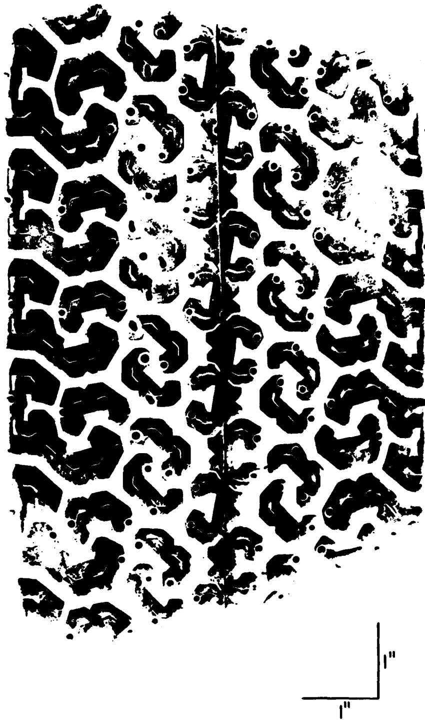
Figure A8. Footprint of tire V at 165 kPa (contact area: 280 cm 2 ).
