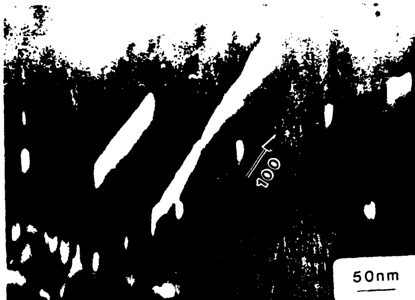
Fig. 19. Weak beam, dark field micrograph of cubic rod shaped particles after isothermal aging for 50 hrs. at 450°C.
