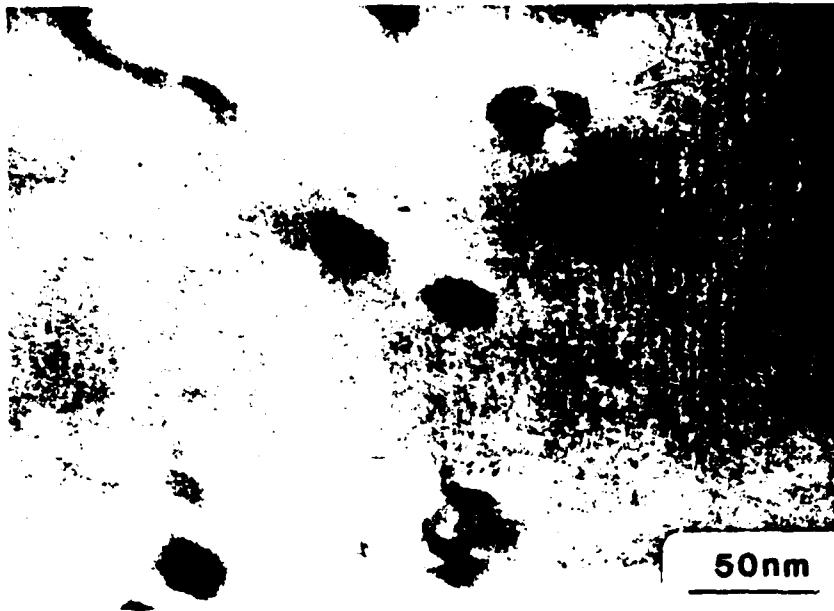
Fig. 13. Bright field micrograph of \text{Al}_3\text{Zr} particles in Al matrix after isothermal aging of 0.5 hrs. at 450^\circ\text{C} .
