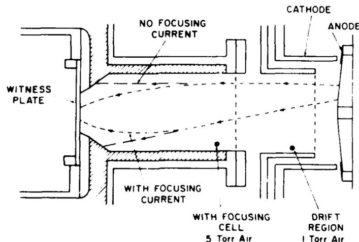
Fig. 3. Schematic of a final-focusing cell.
