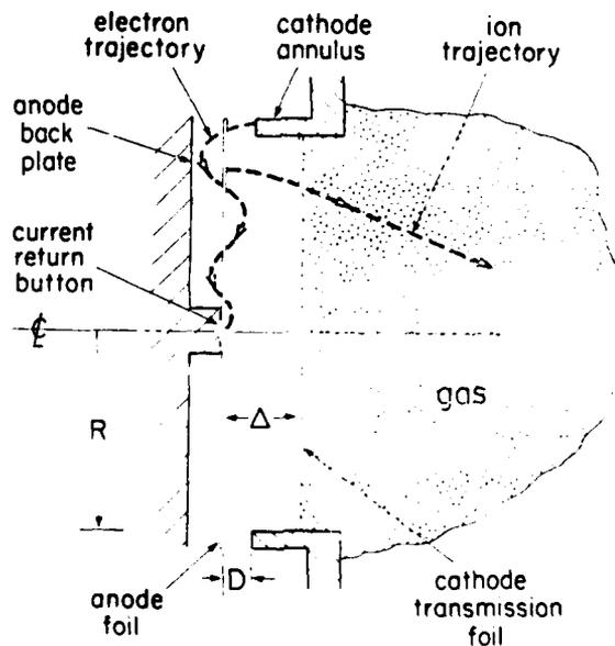
Fig. 2. Schematic of a pinch-reflex diode (PRD).
