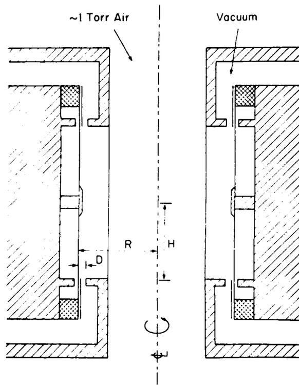
Fig. 4. Schematic of equatorial pinch-reflex diode (EPRD).
