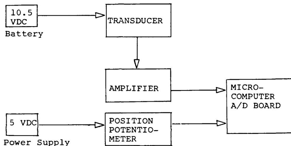
Figure 9. Schematic of Electrical Signal Processing
