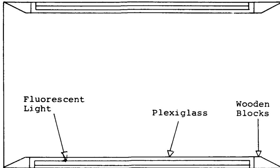
Figure 3. Lighting Modifications to Smoke Tunnel Test Section
