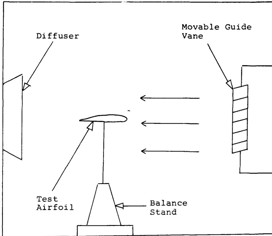
Figure 1. Schematic of Kramer Experiment
