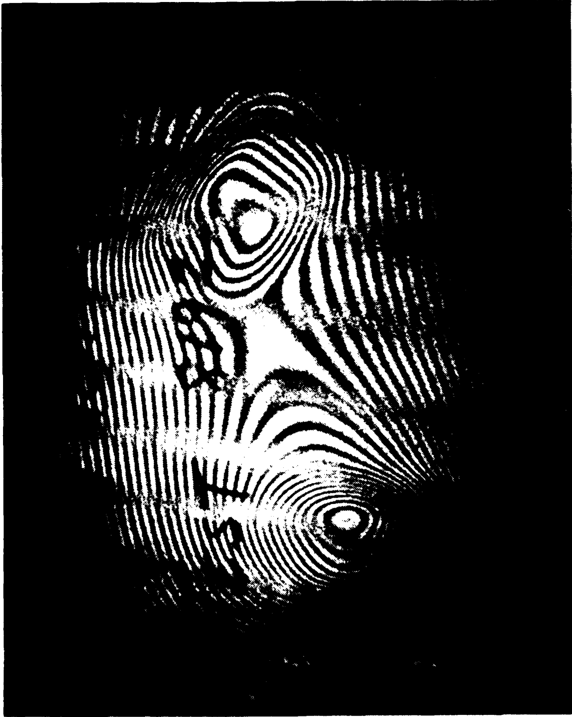
Figure 4-12. Moiré of the Two Random Noise Interferograms Indicating the Presence of the Linear Fringe
