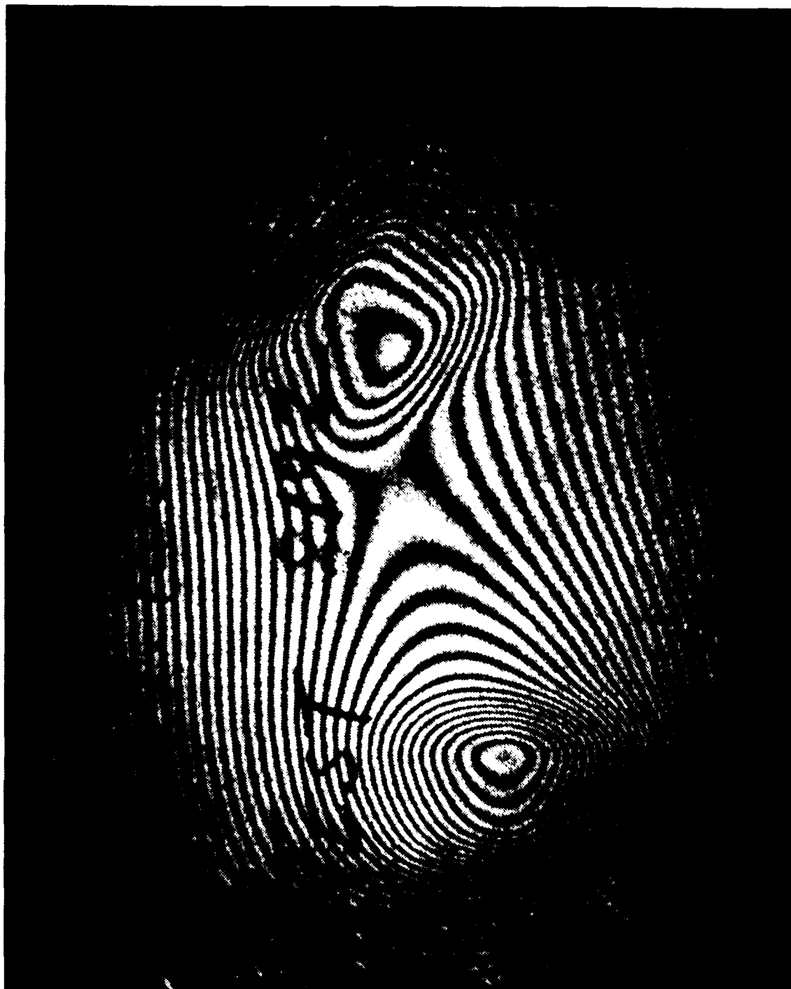
Figure 4-10. Reconstructed Image (Holographic Interferogram) from Double Exposure Hologram #1
