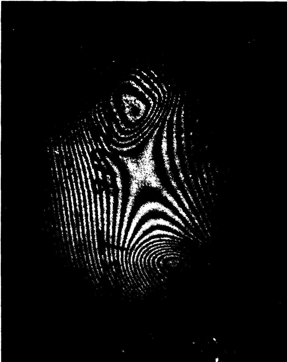
Figure 4-11. Reconstructed image (Holographic Interferogram) from double exposure hologram #2. The linear fringe is not observable.
