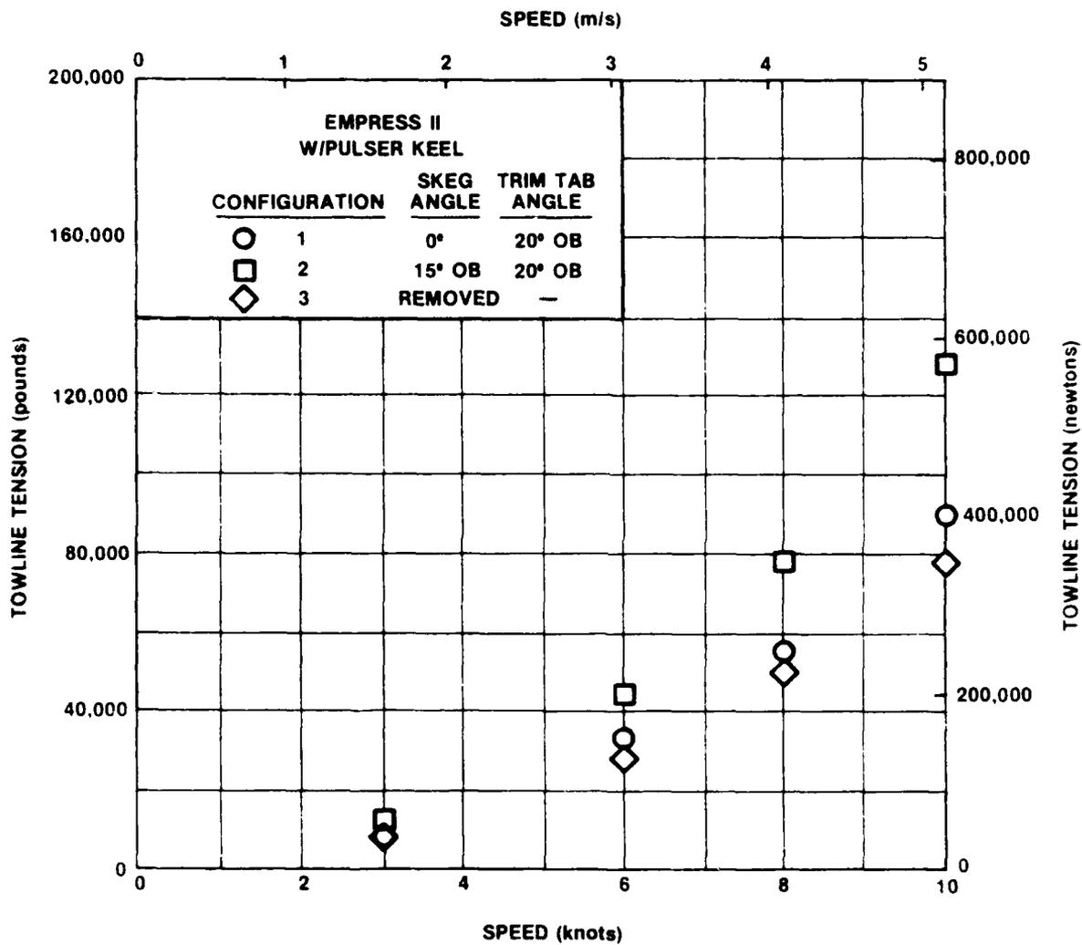
Figure 15 - Towline Tension as a Function of Speed for Various Skag Angles for the EMPRESS II Barge with Pulser Keel
