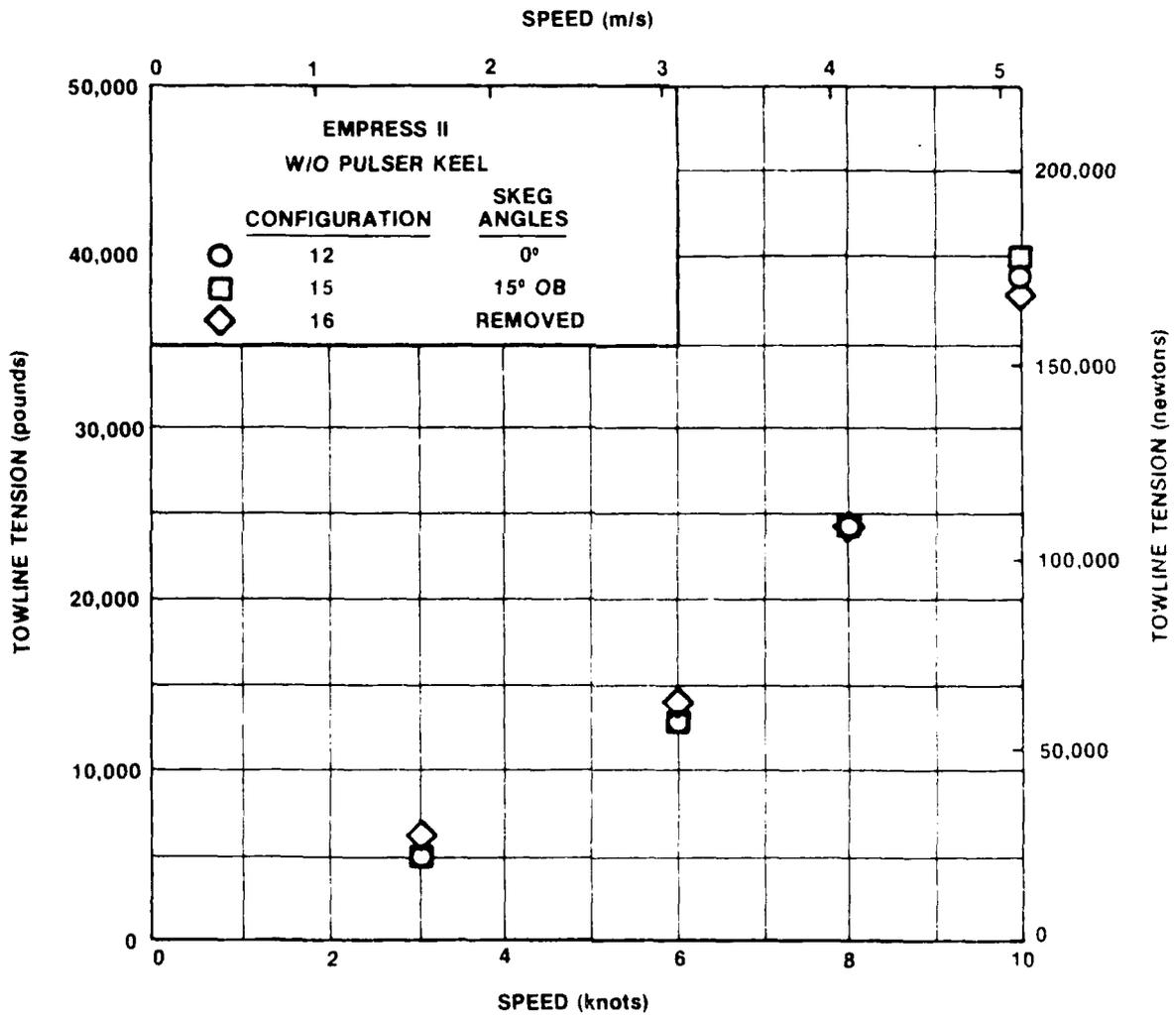
Figure 16 - Towline Tension as a Function of Speed for the Various Skag Angles for the EMPRESS II Barge without Pulser Keel
