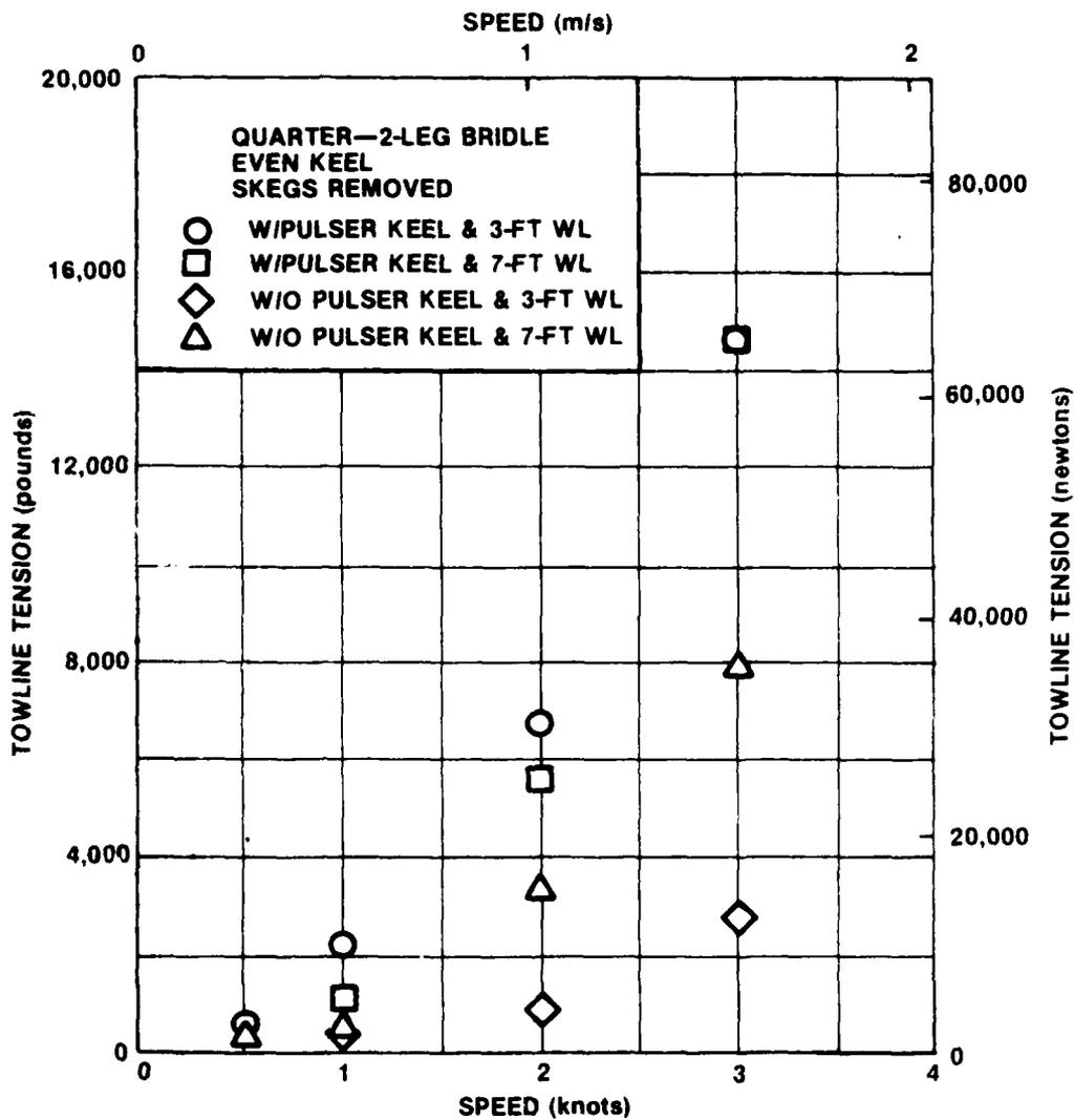
Figure 24 - Mooring Loads as a Function of Speed for 2-Leg Bridle from the Quarter
