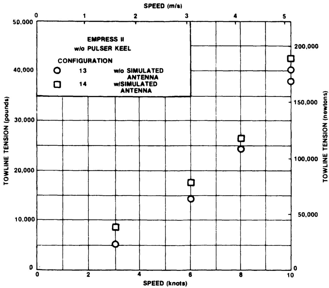
Figure 21 - Towline Tension as a Function of Speed with and without the Simulated Antenna
