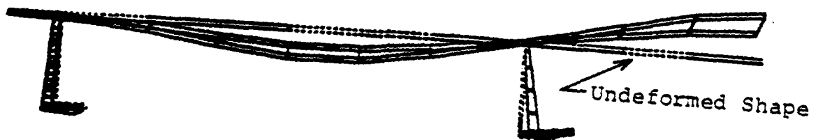
Figure 2.5. Mode 3,3 of Stiffened Panel (120.1 Hz).
