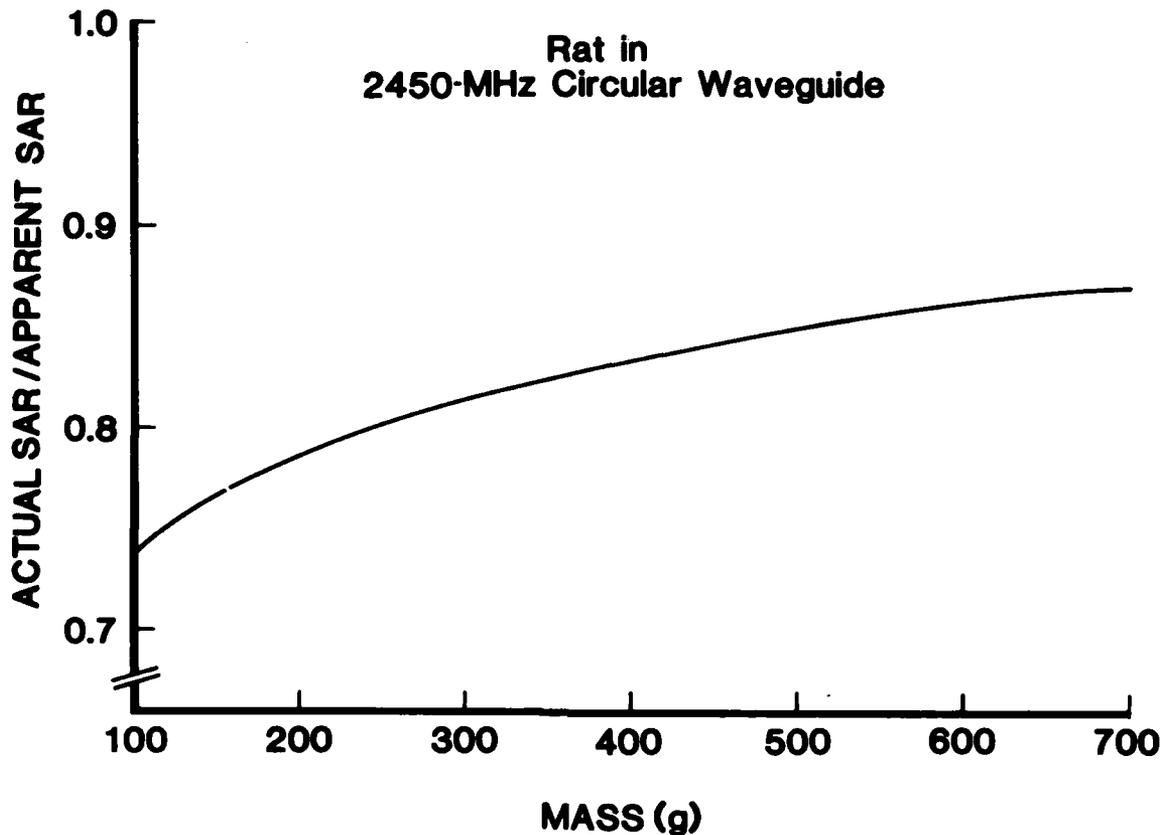
Figure 13. SAR correction factor (actual SAR/apparent SAR) as a function of mass based on average of five positions.
