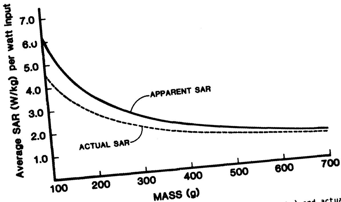
Figure 12. Averages of apparent (five-power-meter measurements) and actual (twin-well calorimeter measurements) SARs for all five positions for exposed animals in waveguide for 1-W input power.
