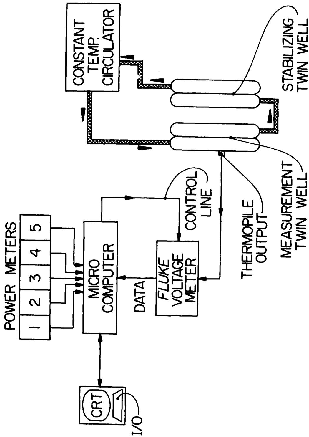
Figure 4. Diagram of the twin-well calorimetry system.
