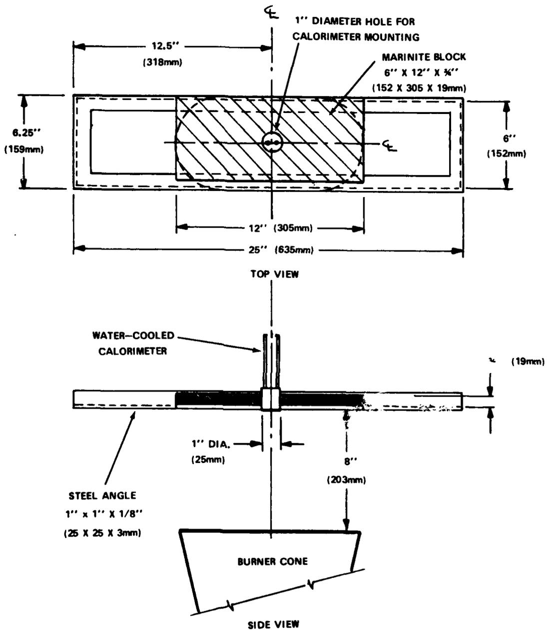
**CALORIMETER BRACKET (SERIES TWO - HORIZONTAL/VERTICAL SAMPLE MOUNTING)**
