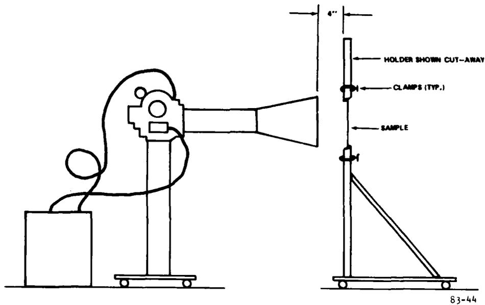
FIGURE 4. 2-GALLON/HOUR BURNER WITH VERTICAL SAMPLE MOUNTING
