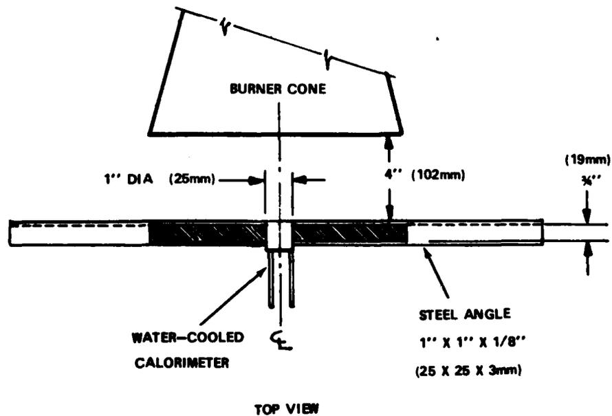
CALORIMETER BRACKET (SERIES ONE - VERTICAL SAMPLE MOUNTING)
