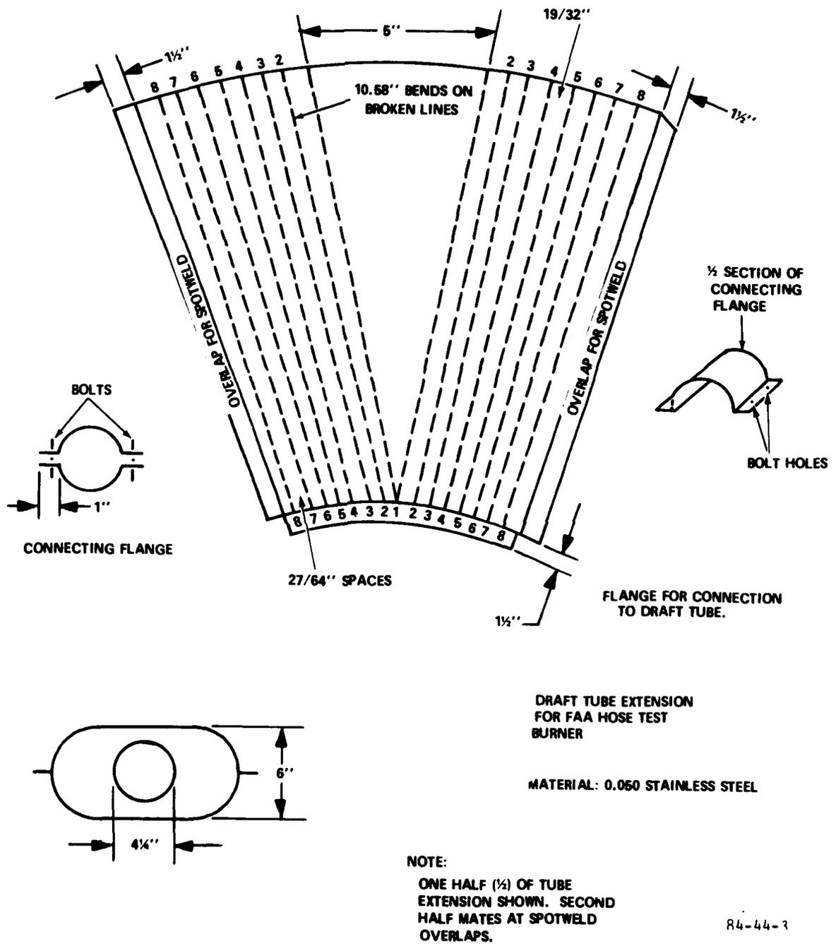
FIGURE 3. DRAFT TUBE EXTENSION FOR FAA HOSE TEST BURNER
