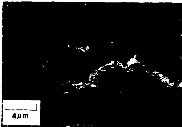
Figure 24. Scanning electron micrographs of shear crack in two-directional carbon-carbon composite
