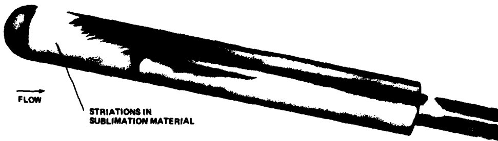
SUBLIMATION MATERIAL ON HEMISPHERE-CYLINDER AT \alpha = 10^\circ , M_\infty = 1.2 , R_{L_\infty} = 4.9 \times 10^6 , L = 7.5 D , D = 2.6 in.
