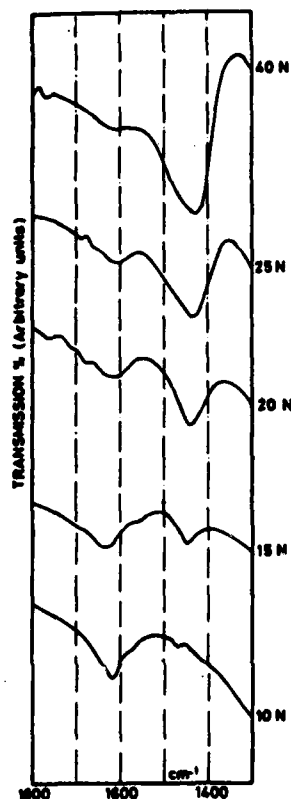
Fig. 5. Evolution of the IR band located at 1450\text{ cm}^{-1} as a function of the \text{Na}_2\text{O} content.
