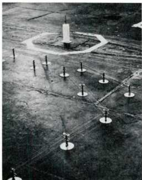
Fig. 33 Photographs of a 600/1 scale model of a power transmission line that runs nearby a MF broadcast antenna. The monopole at the centre of the turntable is surrounded by a styrofoam block to stabilize it against the wind. The upper photograph is a simplified situation; the lower photograph a more complicated model of a real situation.
