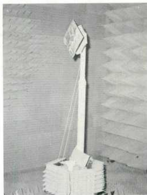
Fig. 12 Antenna under test on a flat plate on positioner (actually this antenna was a cavity backed spiral).
