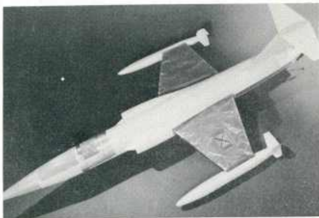
Fig. 11 A 1/12 scale model of a Canadian CF104 fighter aircraft with a crossed slot antenna on the wing.
