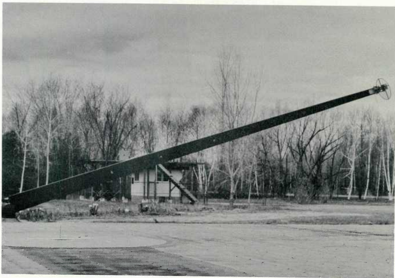
Fig. 2 Photograph of the NRC ground level antenna pattern range showing the boom for measuring elevation patterns and the turntable with a 200 MHz inverted-V dipole antenna on it.
