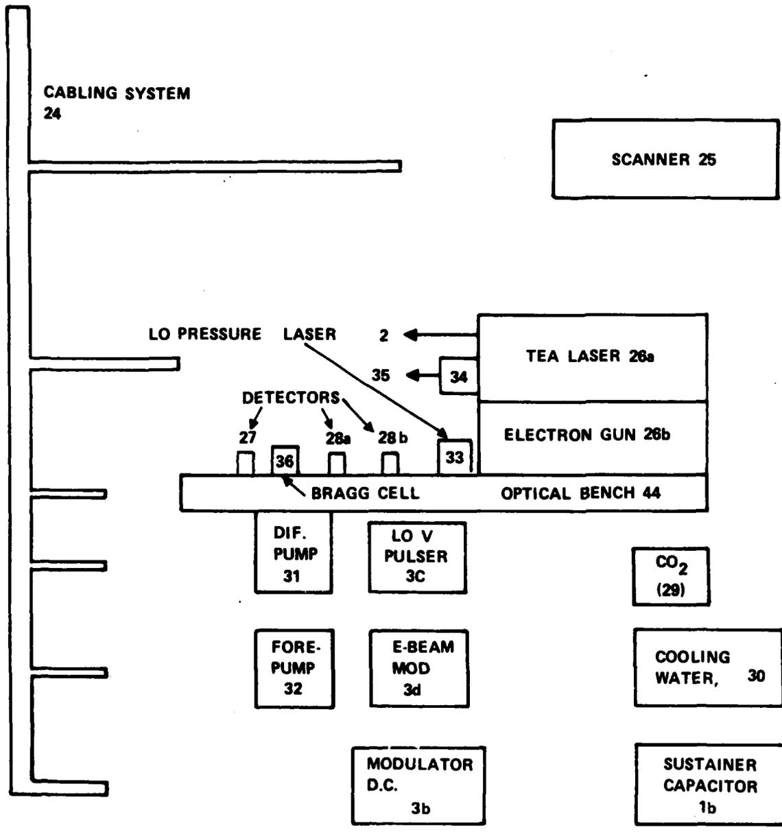
Figure 5b. Electrical System Located at Optical Bench
