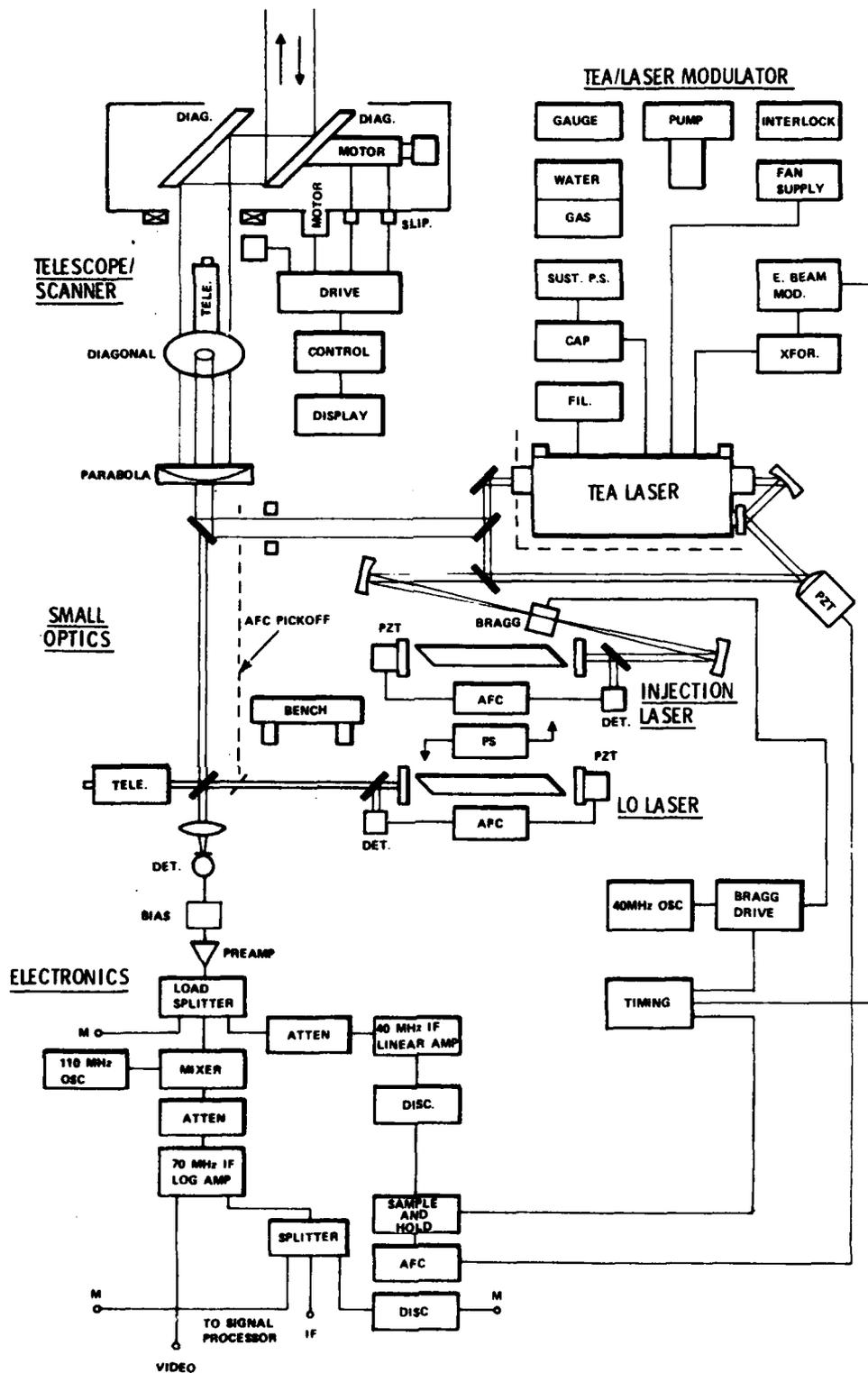
Figure 1. Basic Laser Heterodyne Radar System
