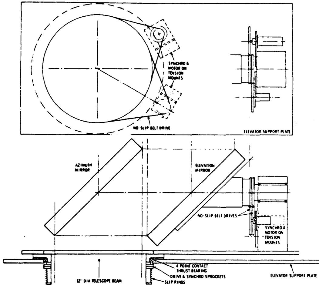
Figure 22. Scanner Bearing Detail
