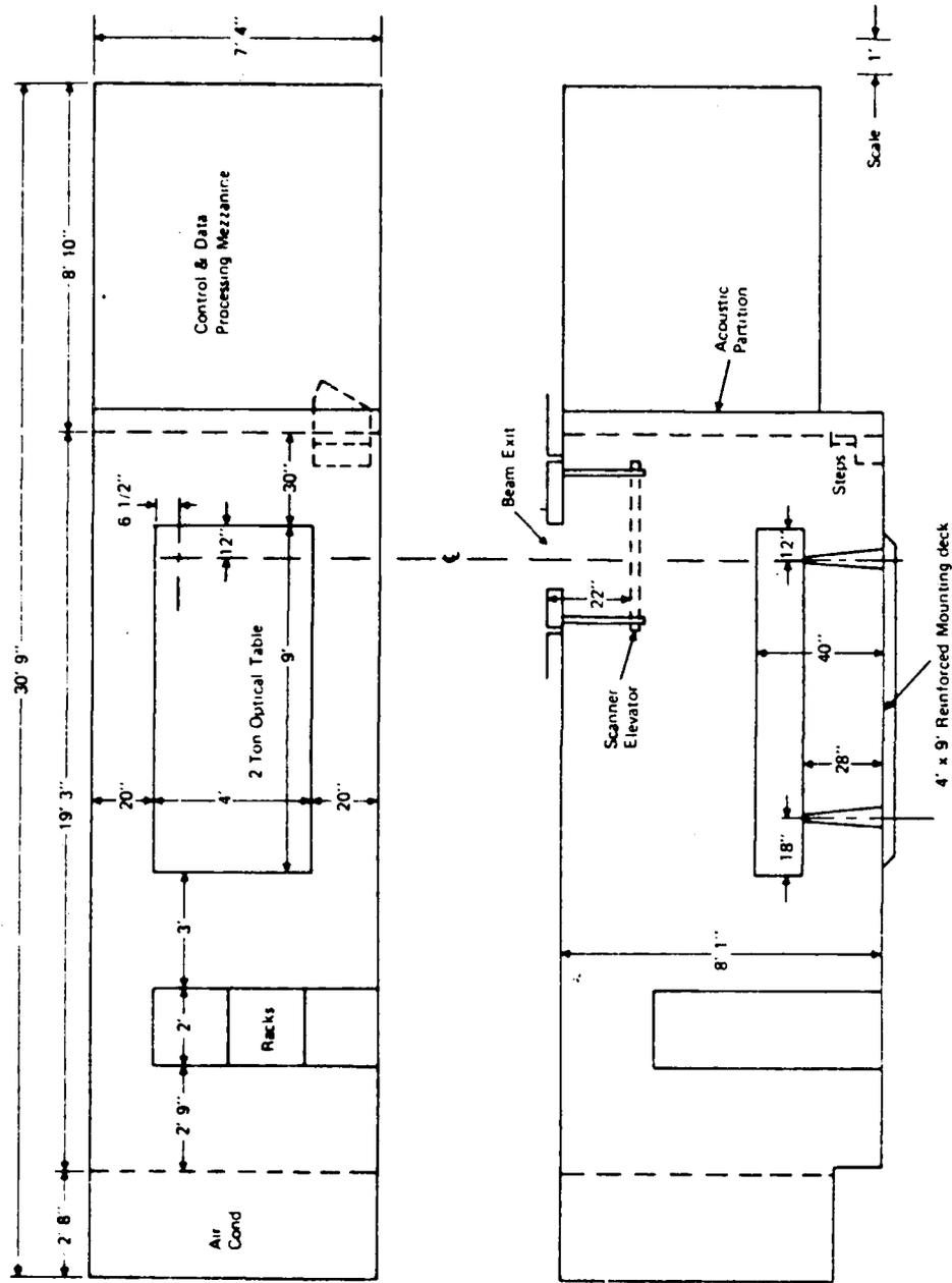
Figure 7. Inside Dimension Requirements.
