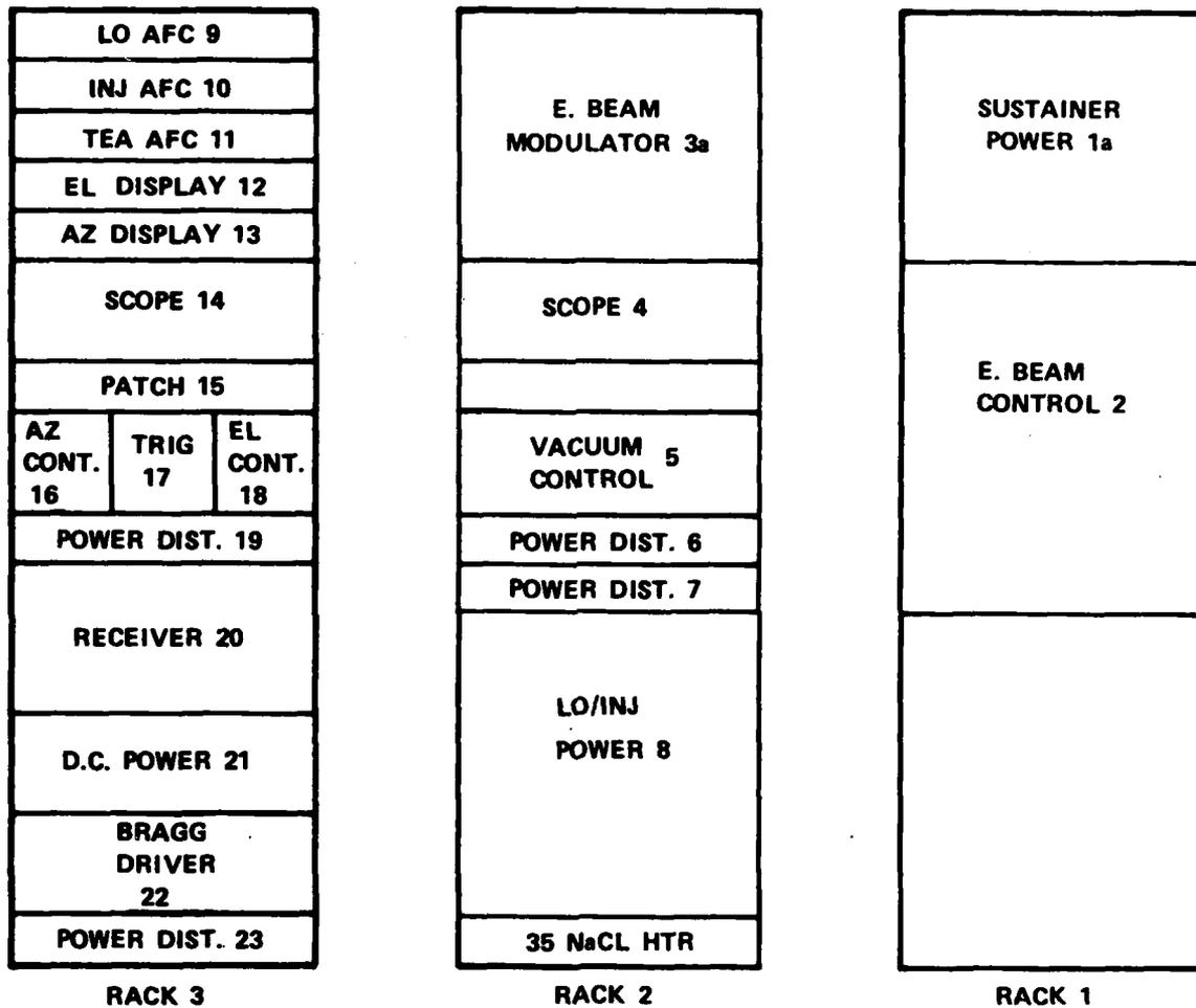
Figure 5a. Electrical System Located in Racks
