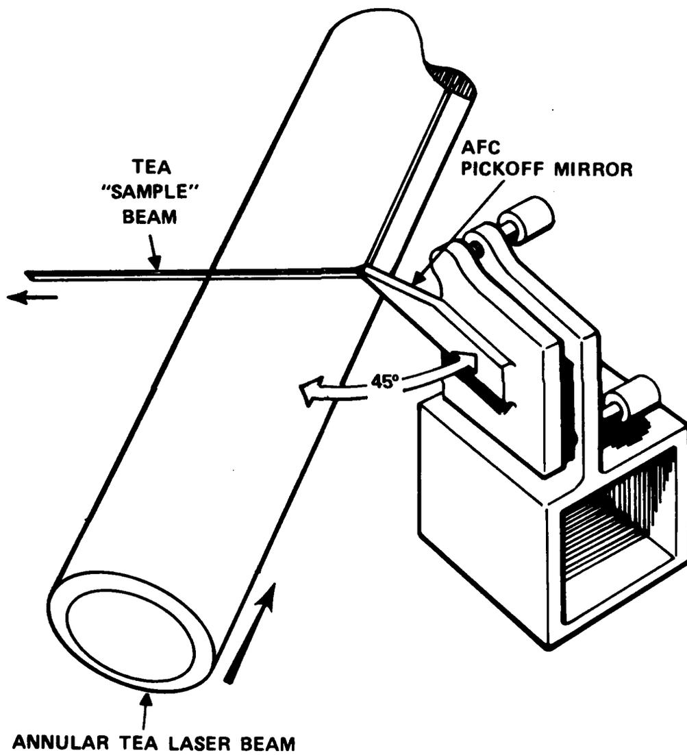
Figure 16. AFC Optical Pickoff, SO #29
