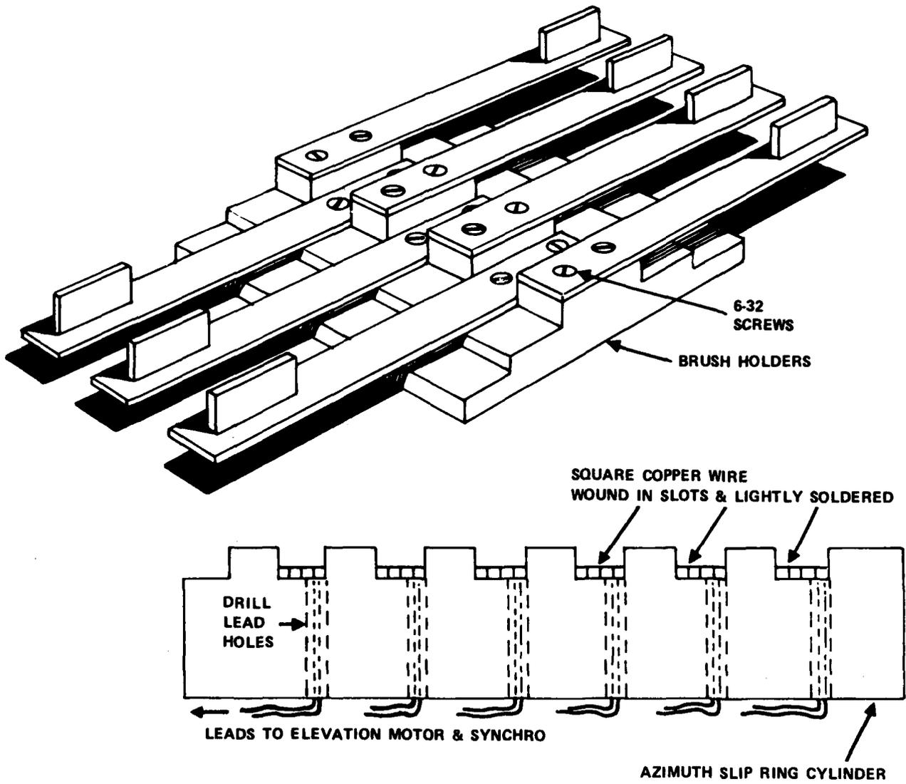
Figure 23. Azimuth Shaft Slip Ring Assembly
