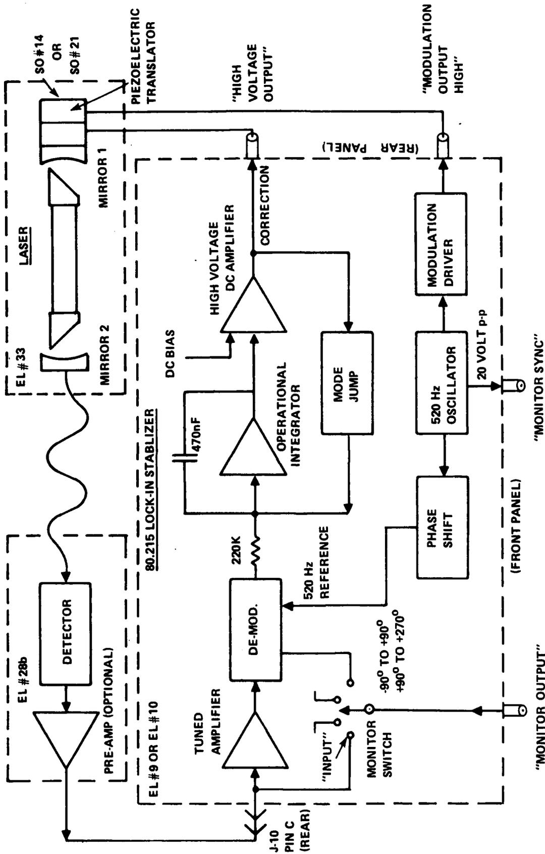
Figure 36. Block Diagram: Stabilized Laser System, Employing 80.215 Lock-in Stabilizer for EL #9 and EL #10
