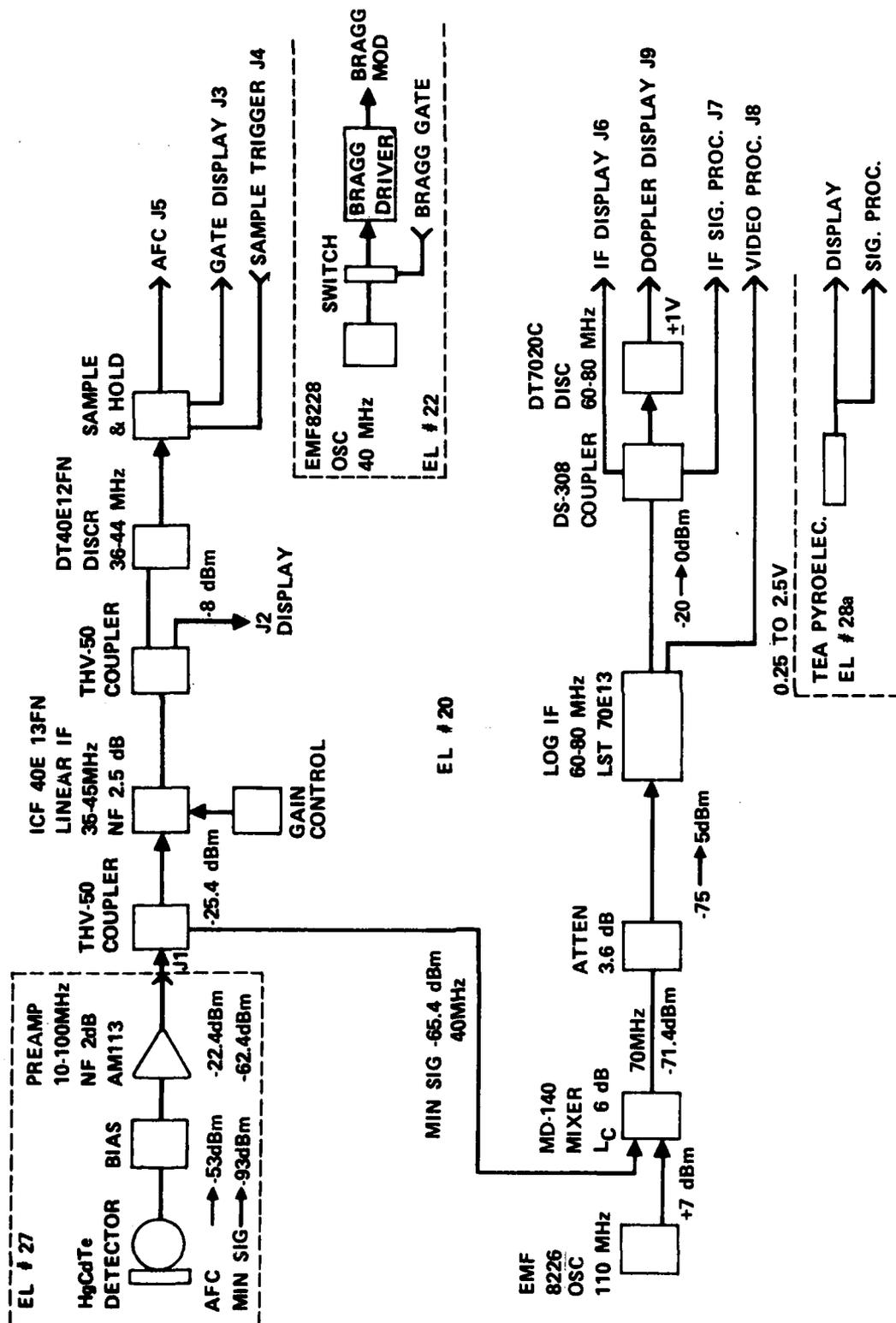
Figure 47. Receiver Electronics, EL #20
