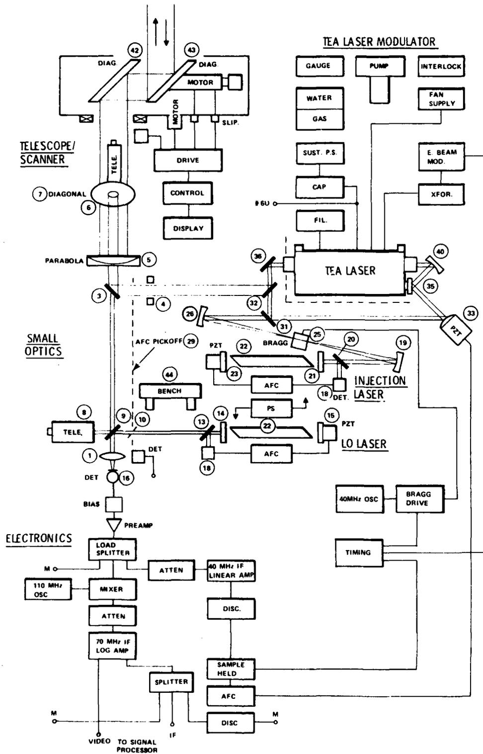
Figure 4. Functional Location of Numbers (SO) Optical Components
