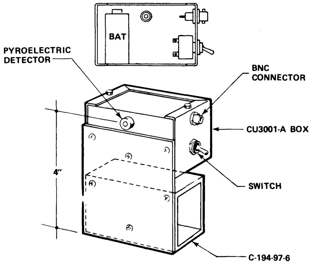
Figure 11. Single Pyroelectric Detector Station #27
