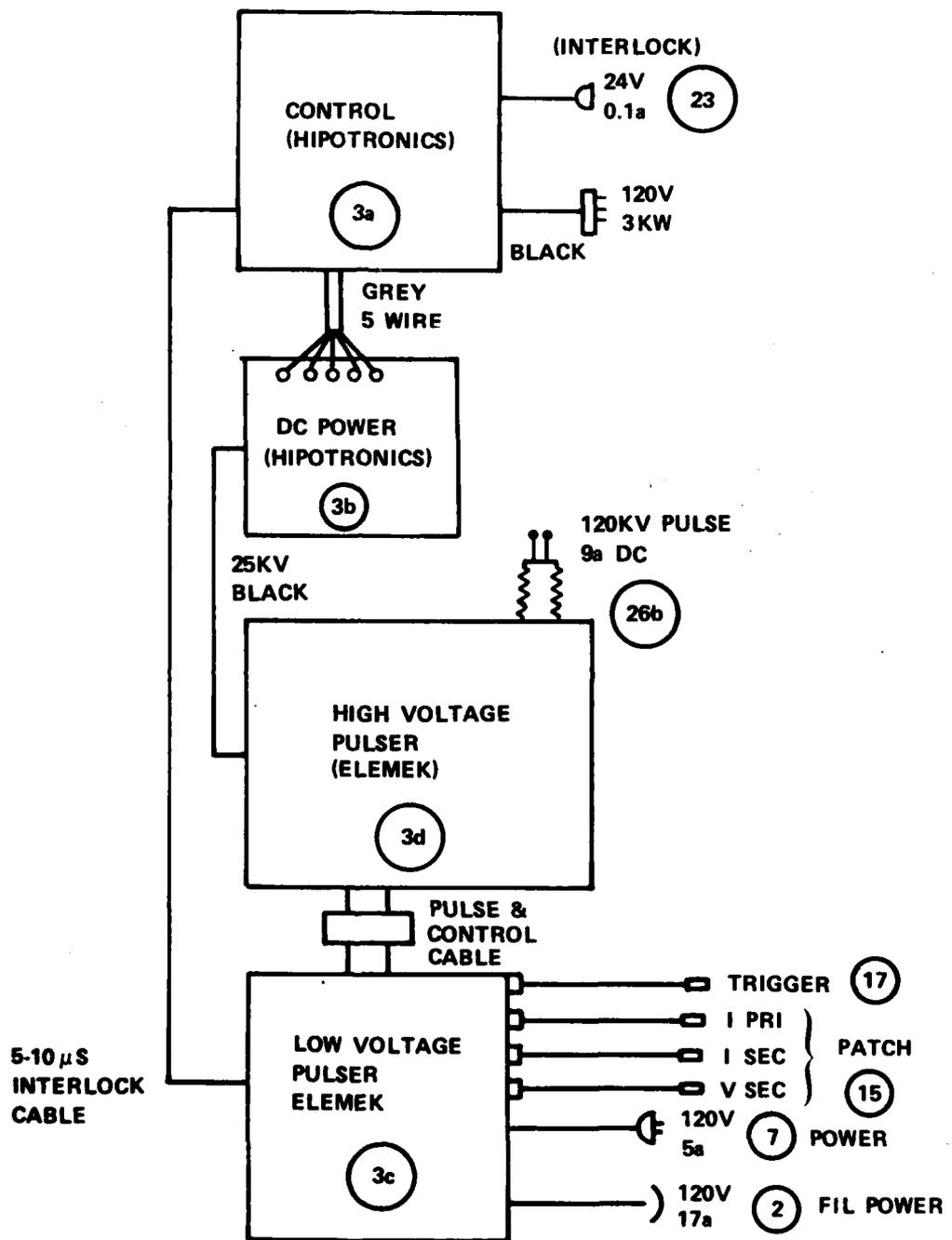
Figure 31. E-Beam Modulator Cabling
