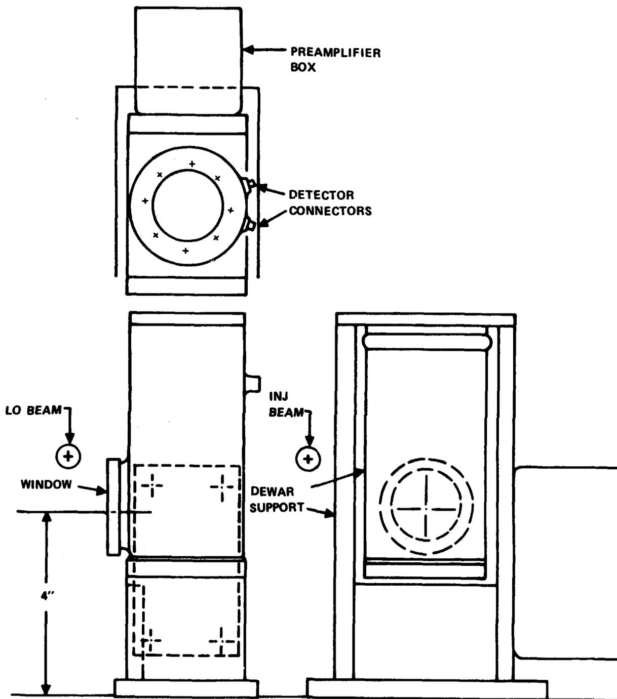
Figure 9. Cryogenic Detector, SO #16
