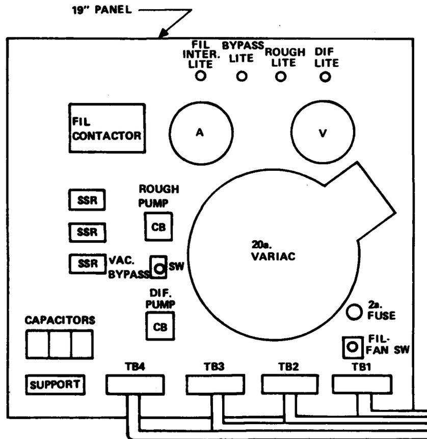
Figure 30. E-Beam Control Panel EL #2
