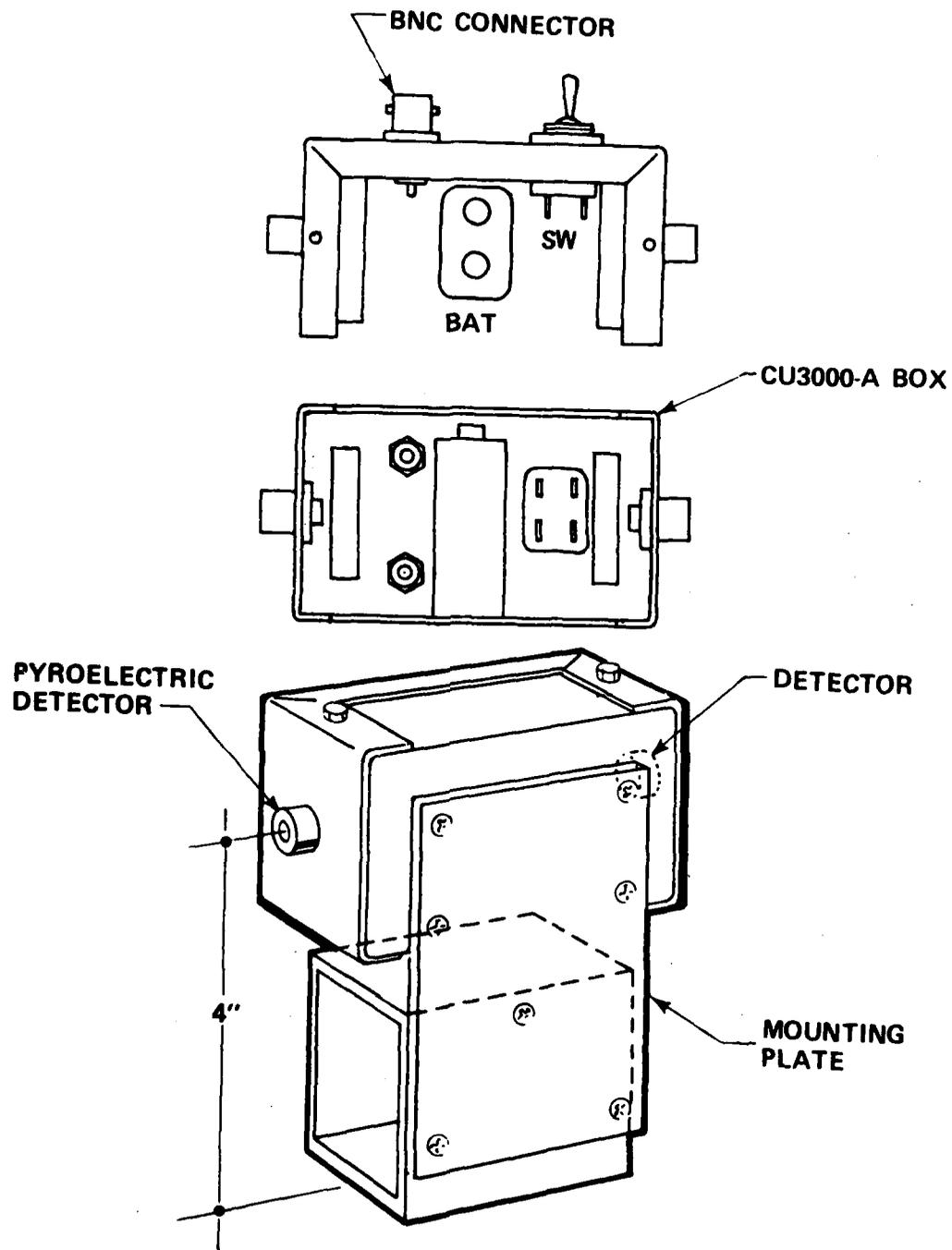
Figure 10. Dual Pyroelectric Detector Station #18
