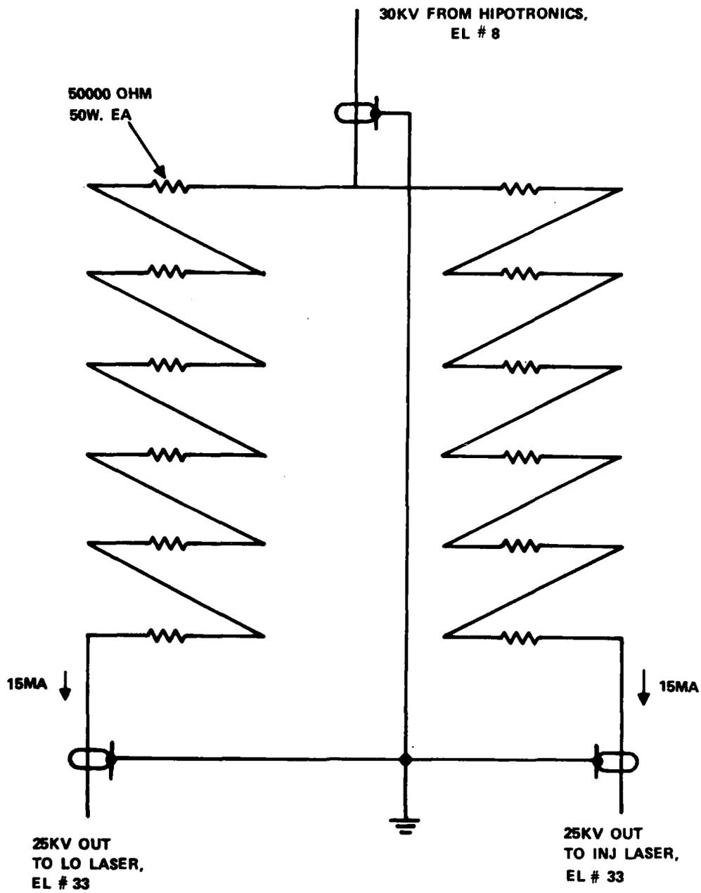
Figure 35. Ballast for Low Pressure CO<sub>2</sub> Lasers, EL #8
