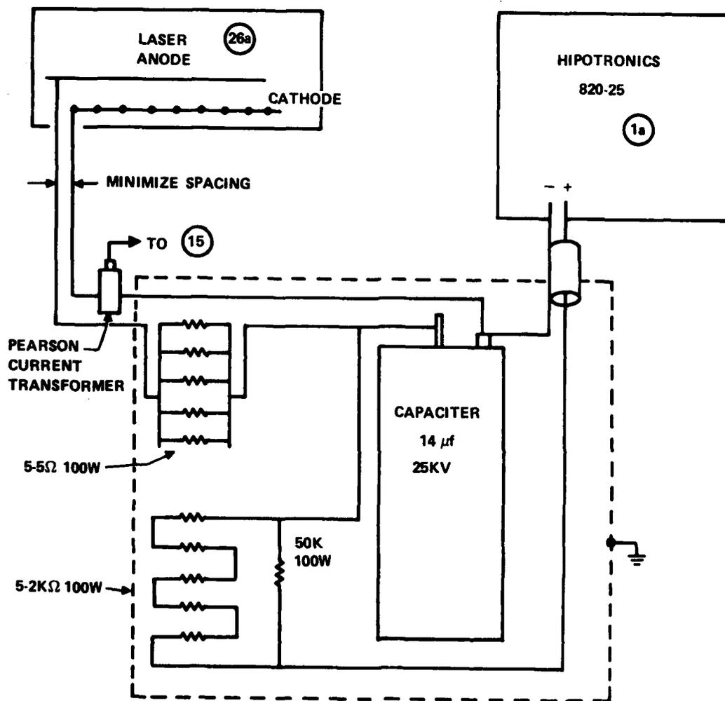
Figure 28. Sustainer Capacitor Ballast and Limiter, EL #1b
