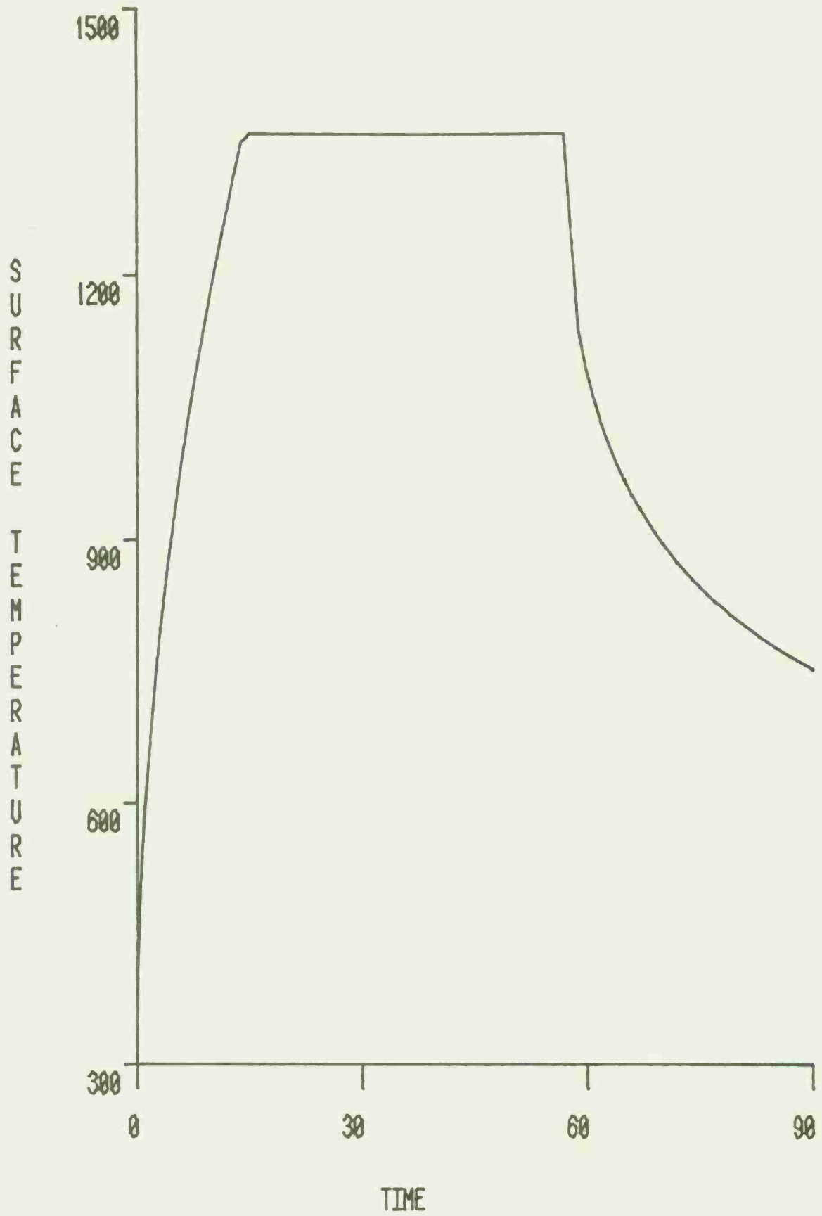
Figure 3. Surface temperature vs. time. The time scale is in microseconds.
