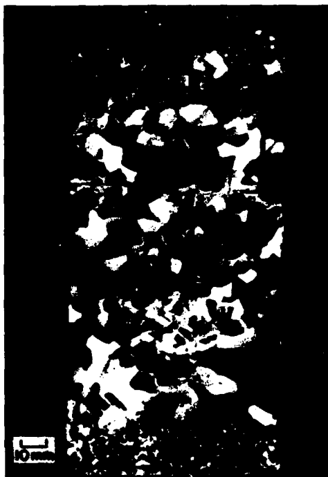
Figure 15. Longitudinal thin section of large-grained sample with refined end zones, after fracture. Note equiaxed, randomly oriented crystal structure in this plane as well, sharp transitions between gauge length and fine-grained ends, and fracture through sample in gauge length.
