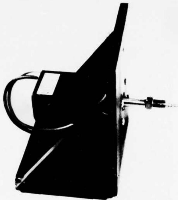
*FIG 1-ACC. CALIBRATION FIXTURE*
