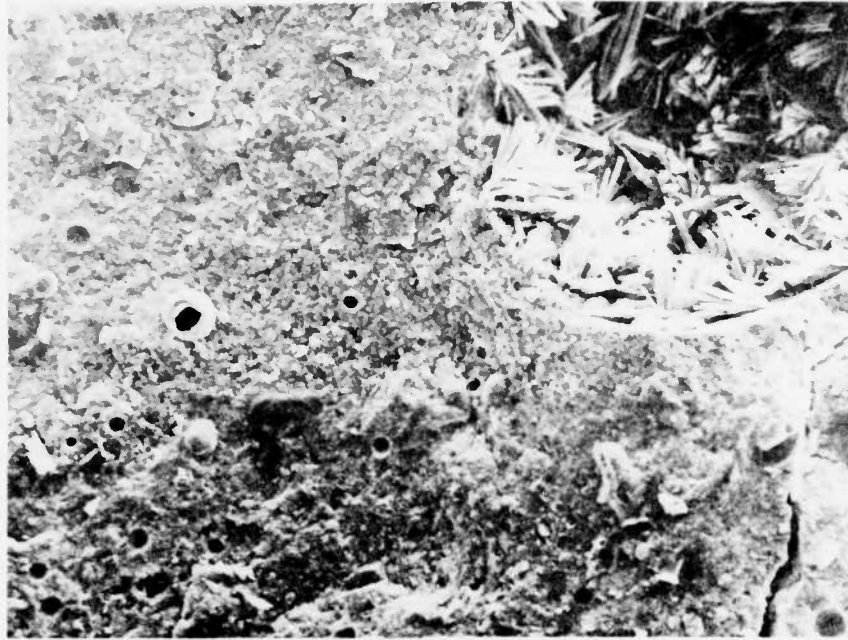
Figure 23. Micrograph 072881-5, X 200. Fracture surface of Mixture M-8-C at 1-year age. Contains shrinkage-compensating cement. Most of field shows typical structure for mature cement paste. The void contains ettringite rods and calcium hydroxide plates.
