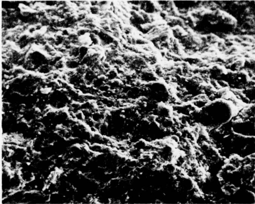
Figure 19. Micrograph 080680-18, X 200. Fracture surface of Mixture M-9-C at 7-day age. The larger size of the AD-628 fly ash spheres is shown by comparison with Figure 20 containing AD-629.
