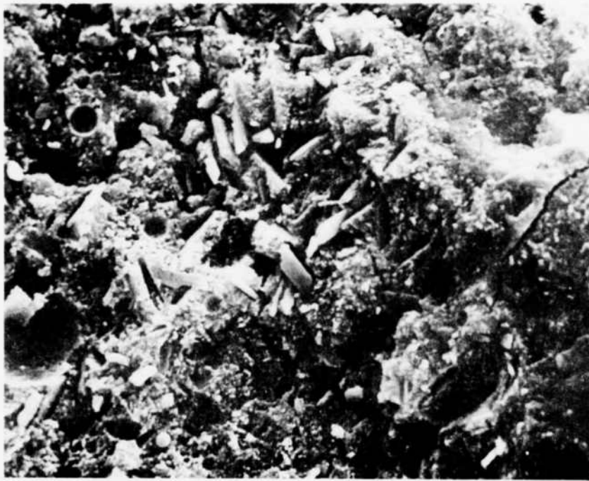
Figure 9. Micrograph 080980-3, X 2000. Fracture surface of Mixture M-9-F at 3-day age. The many elongated platy crystals are believed to be hydrous calcium sulfate from the expansive additive (AD-626). The elongated voids in this and the next micrograph (Figure 10) are believed to be imprints of these crystals.
