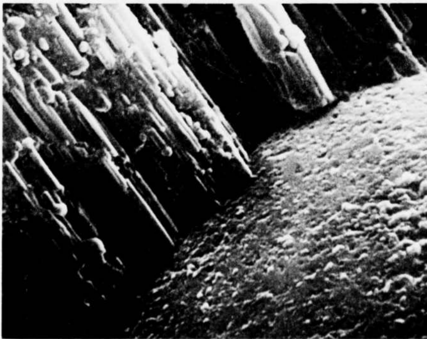
Figure 11. Micrograph 090380-5, X 5000. Fracture surface of Mixture M-9-F at 28-days age. Broken fly ash sphere with a piece of hydration debris from the fracture surface in it. More of these spheres seem to fracture through rather than at the paste to sphere contact as hydration progresses.
