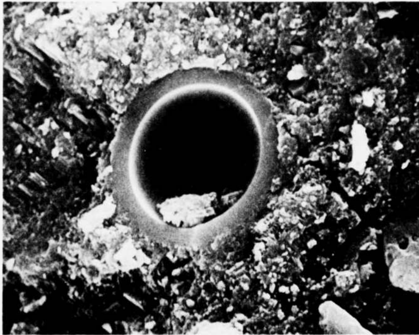
Figure 11. Micrograph 090380-5, X 5000. Fracture surface of Mixture M-9-F at 28-days age. Broken fly ash sphere with a piece of hydration debris from the fracture surface in it. More of these spheres seem to fracture through rather than at the paste to sphere contact as hydration progresses.
