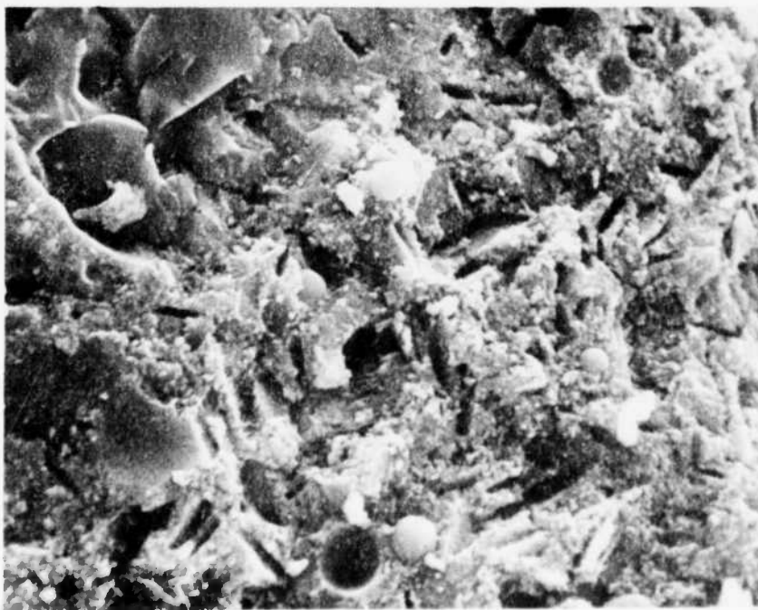
Figure 9. Micrograph 080980-3, X 2000. Fracture surface of Mixture M-9-F at 3-day age. The many elongated platy crystals are believed to be hydrous calcium sulfate from the expansive additive (AD-626). The elongated voids in this and the next micrograph (Figure 10) are believed to be imprints of these crystals.
