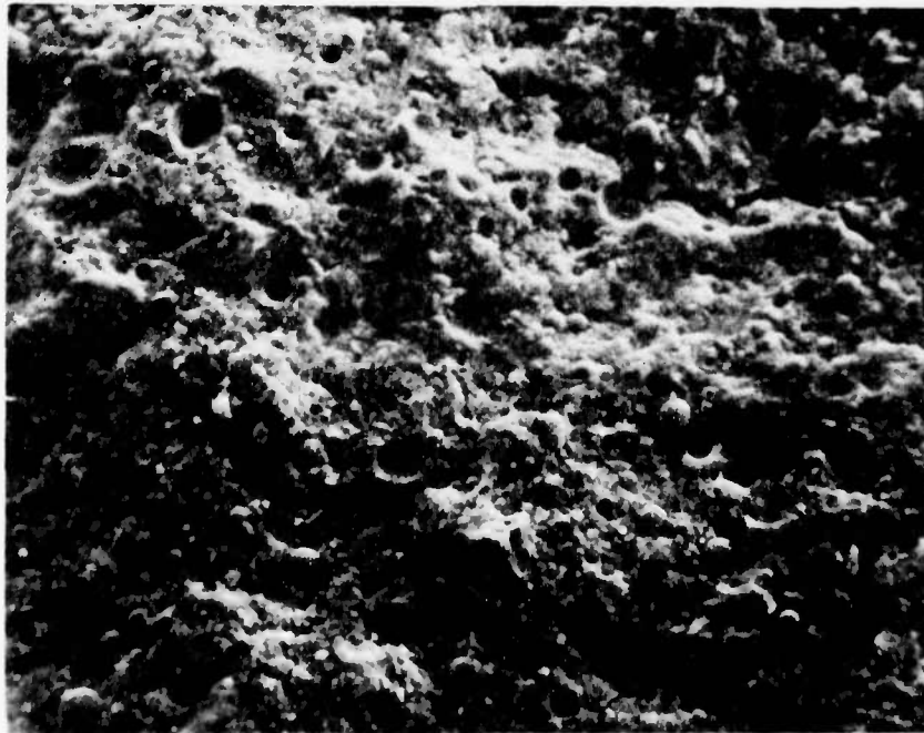
Figure 19. Micrograph 080680-18, X 200. Fracture surface of Mixture M-9-C at 7-day age. The larger size of the AD-628 fly ash spheres is shown by comparison with Figure 20 containing AD-629.
