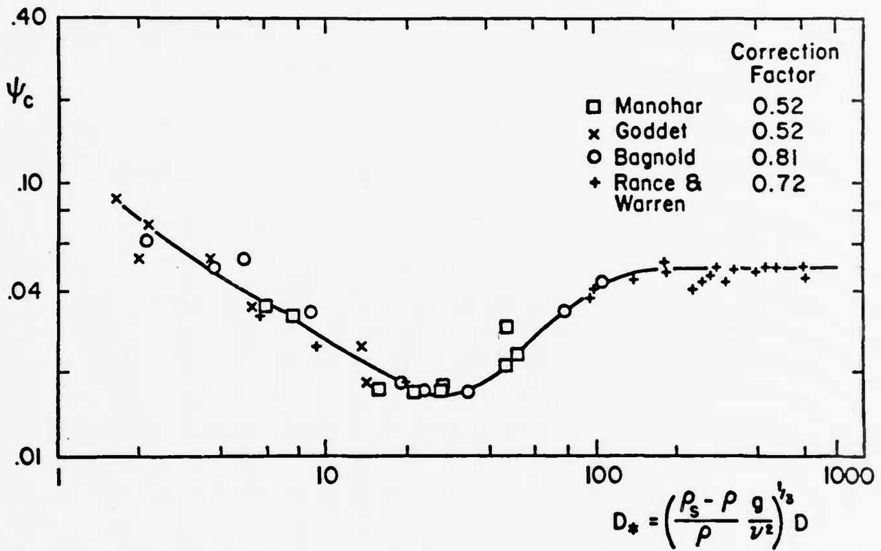
Figure 11. Modified Shields curve for oscillatory flow (Sleath 1978)
