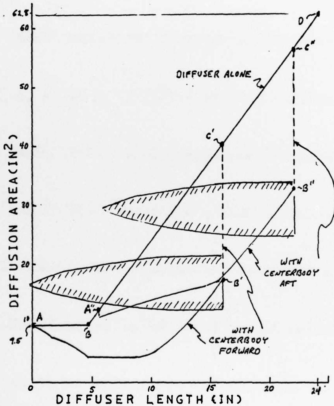
Figure 10. Limiting Cases of Diffuser Area Distributions
