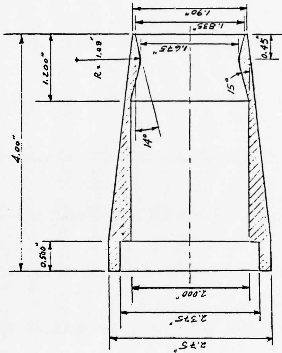
Figure 16. TF30AB Engine Model
