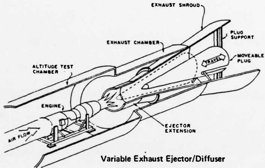
Figure 1. Variable Area Ejector-Diffuser
