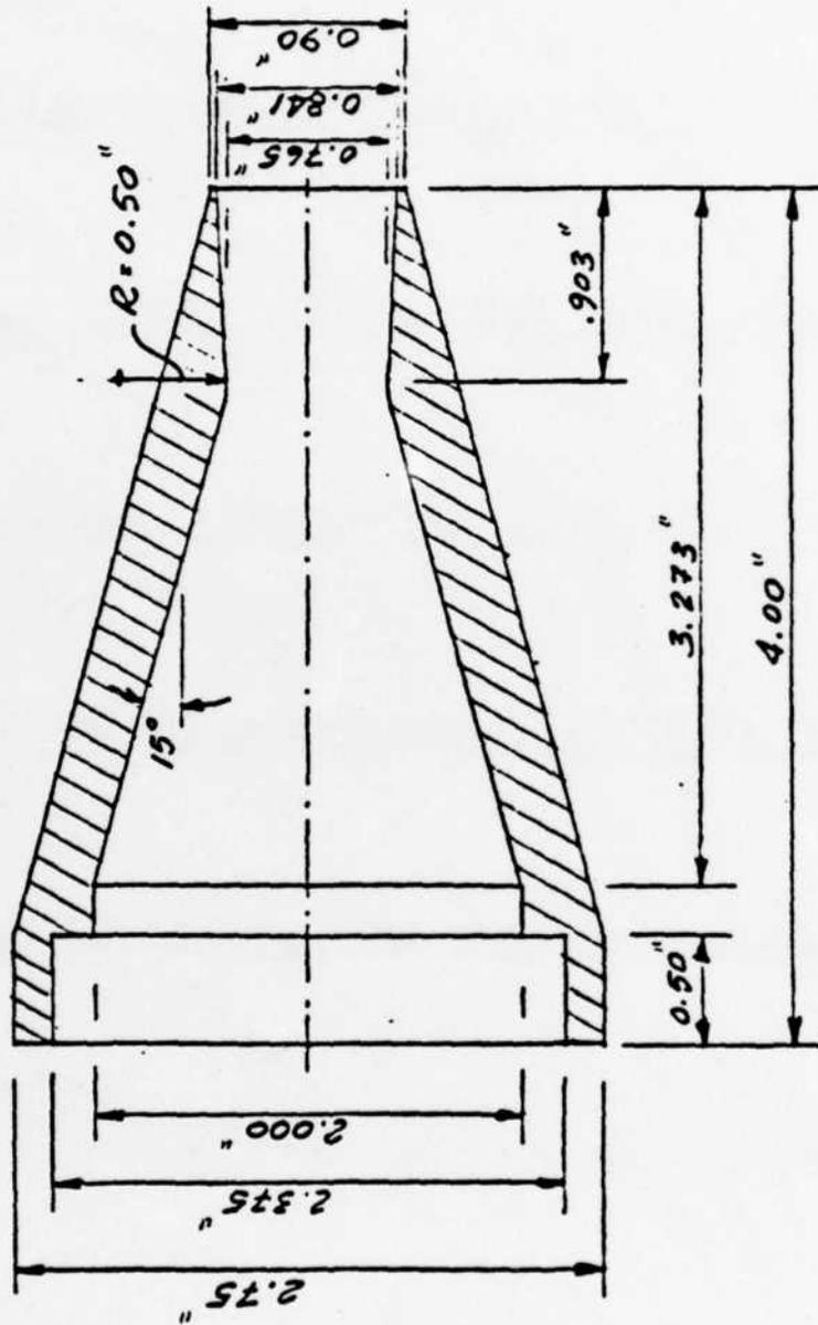
Figure 13. 404NAB Engine Model
