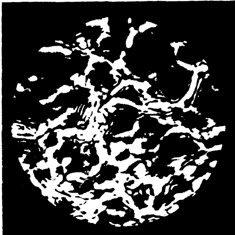
Figure 32. An "open camera" photograph of a scintillating beam profile.
