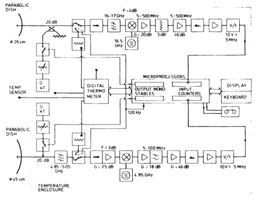
OIL RADIOMETERS 5 GHz, 16.5 GHz
