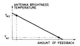
Figure 2. Antenna Brightness temperature as a function of the amount of the feedback value.
