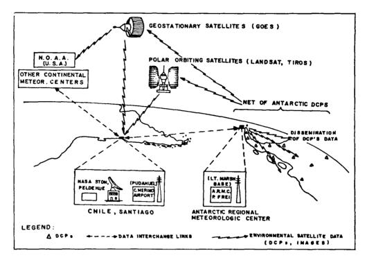
FIG. 3. Operational scheme to collect environmental data from remote sites in Antarctic Penins da by using Satellite Data Collection Systems (DCS).
