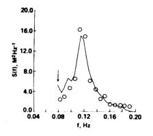
Fig. 17. Comparison of radarinferred (solid line) and buoy (circles) high frequency spectra in absolute units. The arrow indicates the cut-off frequency in order to avoid effects of the antenna pattern at low frequencies. This nondirectional spectrum corresponds to the directional spectrum in Fig. 16.
