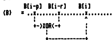
Figure 1: Relationship between bits in a Tausworthe sequence.
