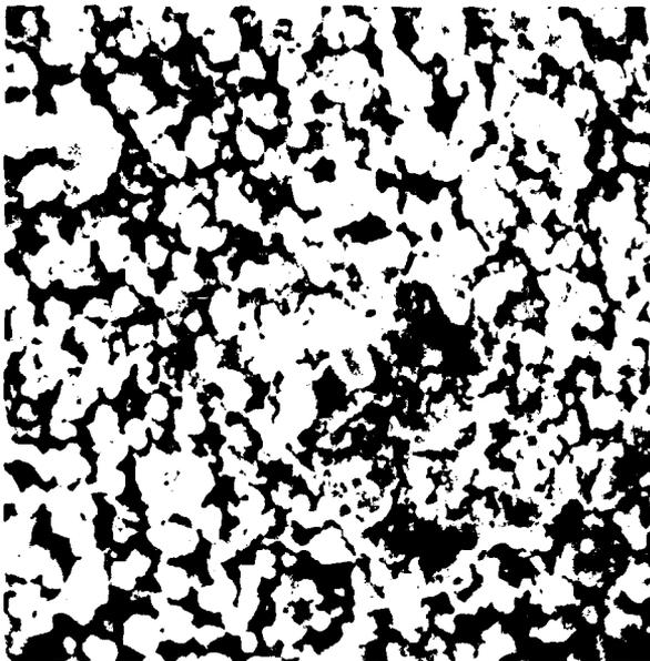
Figure 4. SEM micrograph of a silver deposit on enamel produced by 1 M  $\text{AgF}$  - sat.  $\text{FeSO}_4$  +  $\text{H}_2\text{SO}_4$  (2 pH) (10 repetitions). 3000X.
