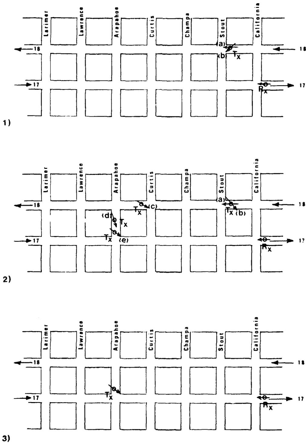
Fig. 3.34 Test locations using the 9.6, 28.8, and 57.6 GHz millimeter wave test system in downtown Denver for non-line-of-sight measurements.
