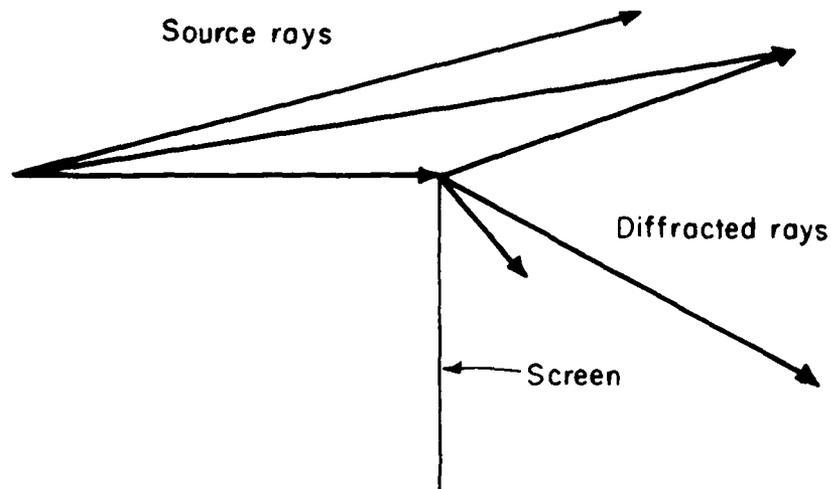
Figure B.3 The ray geometry for Keller's geometrical theory of diffraction.
