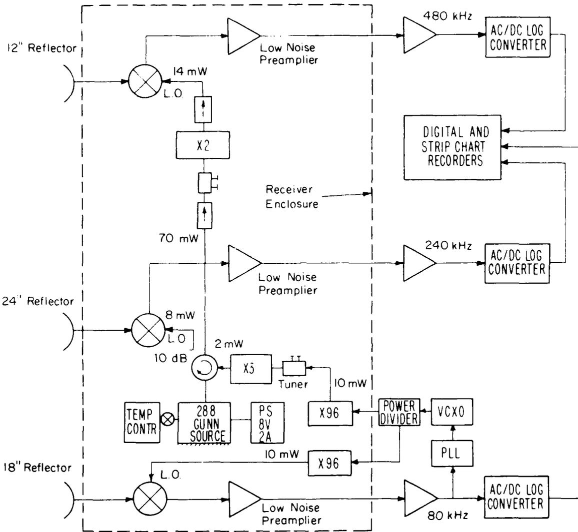
Fig. 2.2 A functional diagram of the receiving terminal.
