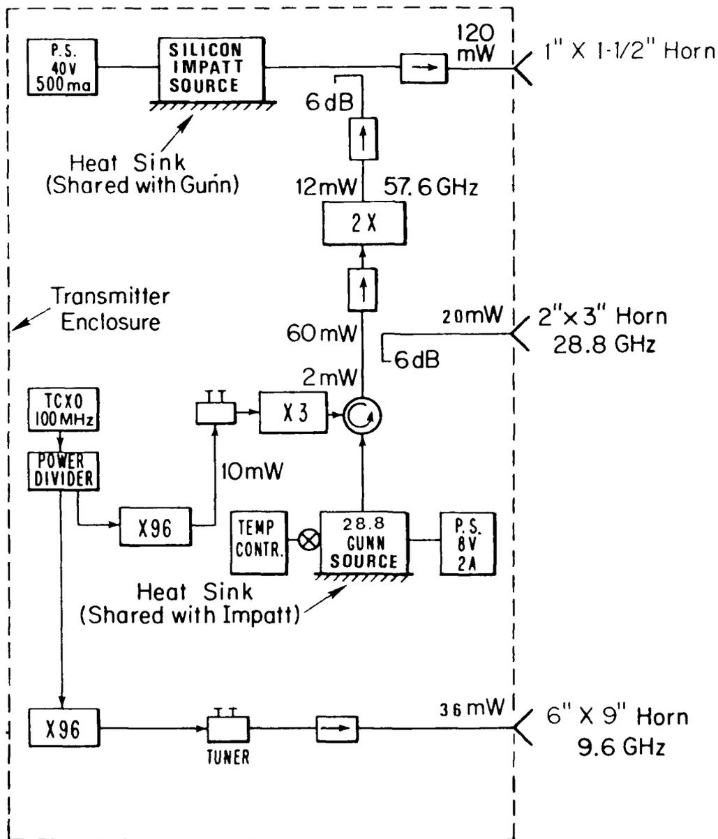
Fig. 2.1 A functional diagram of the transmitting terminal.
