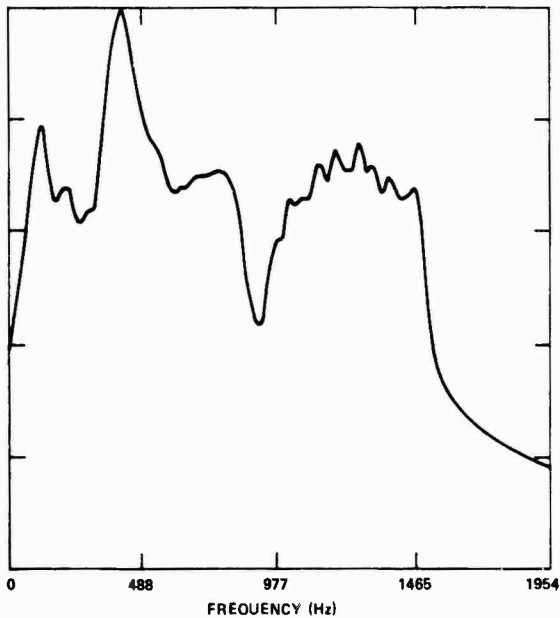
Fig. 13 - P.S.D. curve of response signal of finite element model (Point 1)
