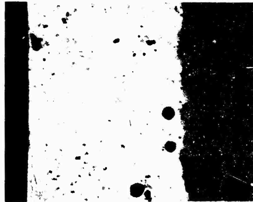
Figure 6: S2-B Enamel Coating on Hastelloy-X Substrate-as Coated
