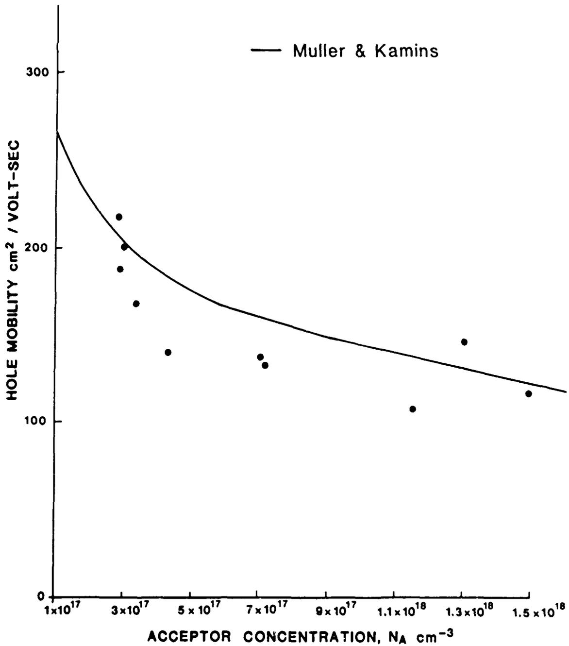
**Fig. 12 HOLE MOBILITY VS. ACCEPTOR CONCENTRATION FOR ALL Ga DOPED SILICON MBE FILMS GROWN AT UCLA TO DATE.**
