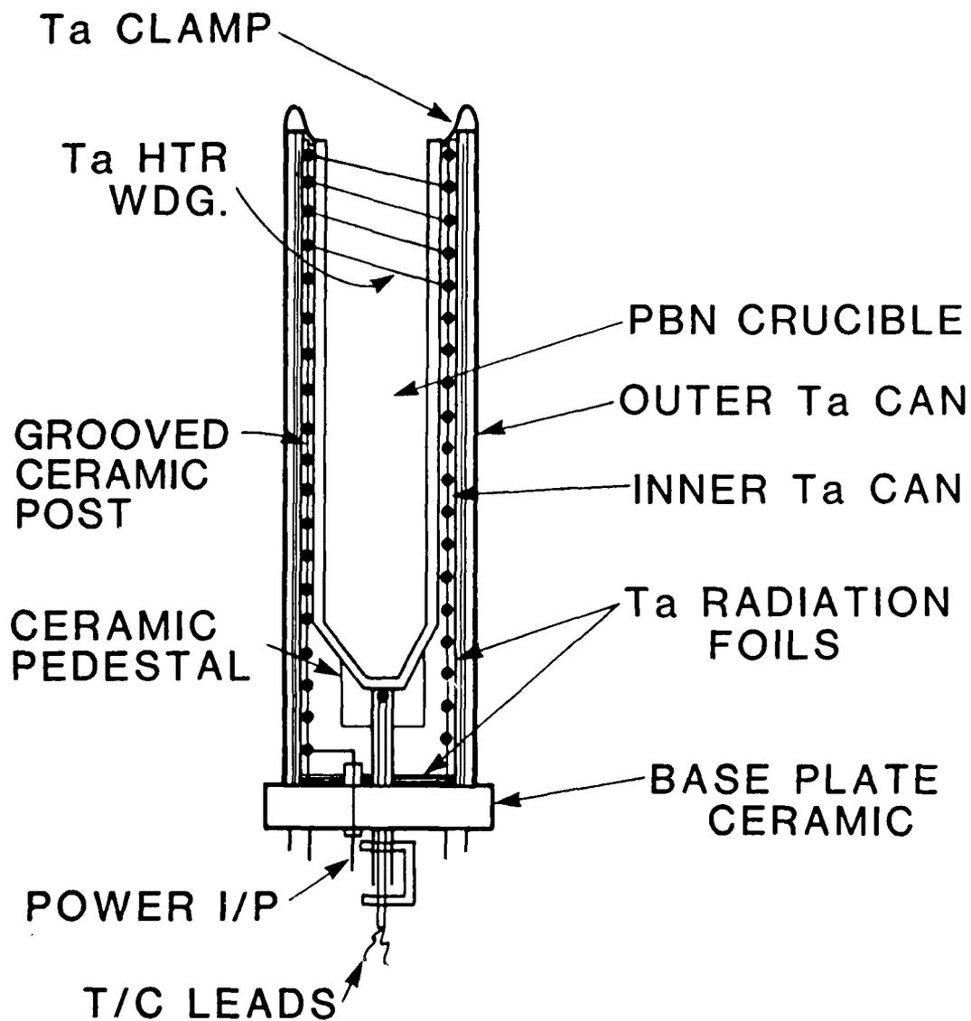
Fig. 3 SCHEMATIC OF UCLA EFFUSION CELLS
