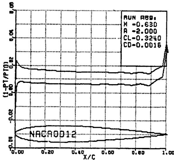
Figure 8. Surface total pressure loss for 65\*17 mesh with reduced skewness near trailing edge.
