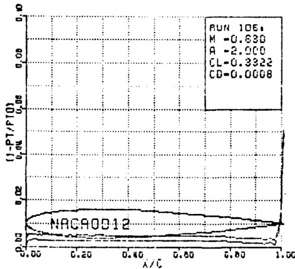
Figure 15. Surface total pressure loss for double embedded leading edge mesh.
