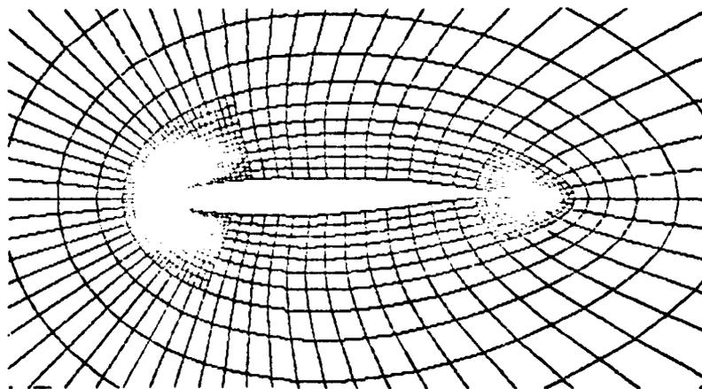
Figure 26. Embedded mesh regions, Korn airfoil for  $M_\infty = 0.75$  and  $\alpha = 0.12$  deg.
