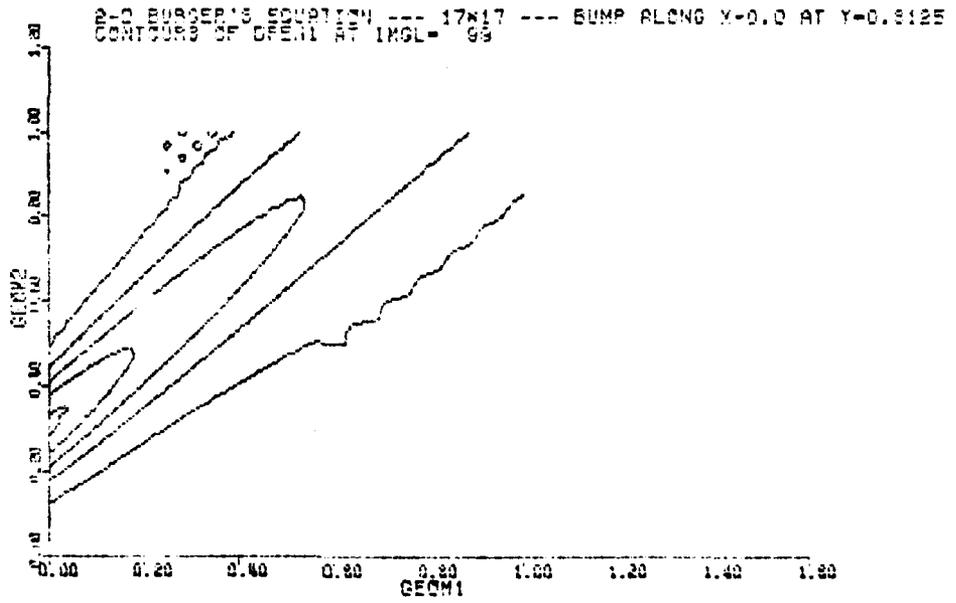
Figure 9 Two-dimensional field contours for model convection/diffusion equation (4)
