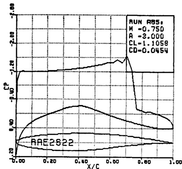
Figure 24a. Surface pressure coefficient.
