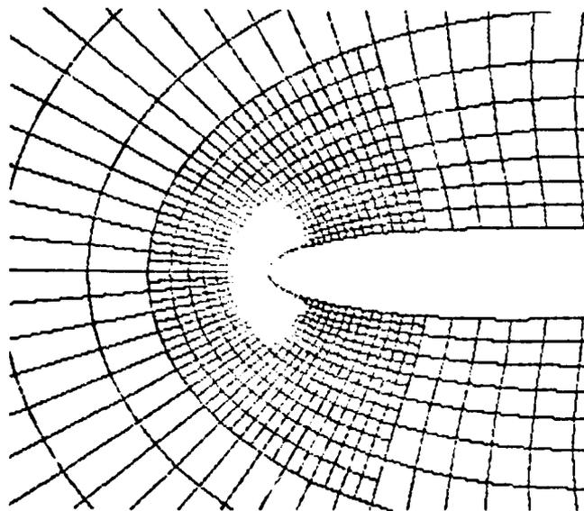
Figure 14. Double embedded mesh in the leading edge region.
