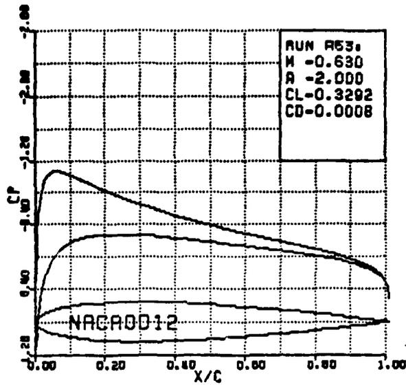
Figure 5a. Surface pressure coefficient.
