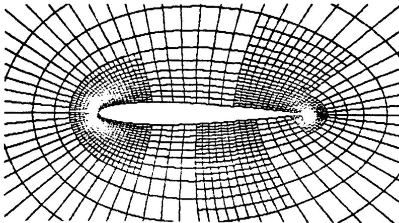
Figure 20. Embedded regions, NACA0012 airfoil for  $M_\infty = 0.85$  and  $\alpha = 1.0$  deg.
