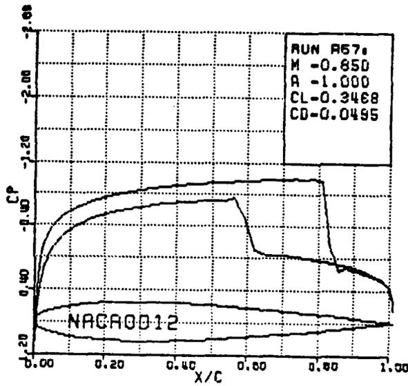
Figure 21a. Surface pressure coefficient.
