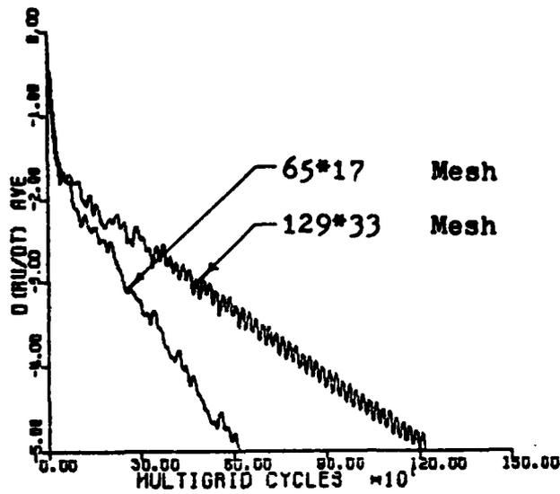
Figure 7. Convergence histories for NACA0012,  $M = 0.63$  and  $\alpha = 2.0$  deg.
