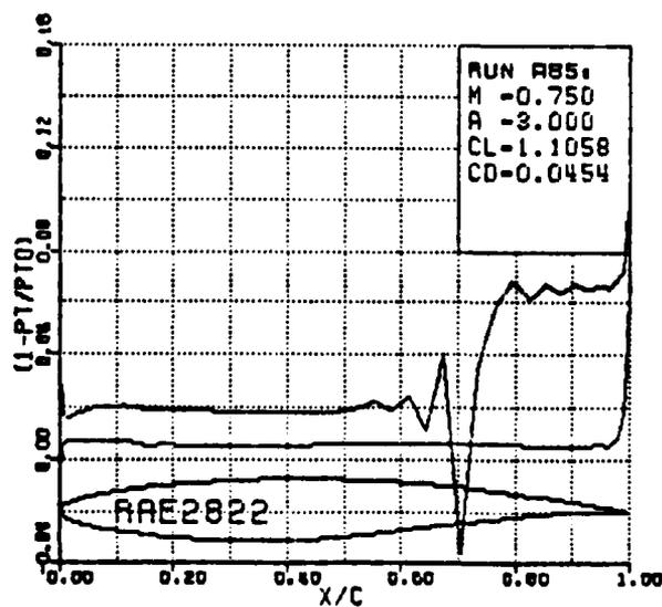
Figure 24b. Surface total pressure loss.
