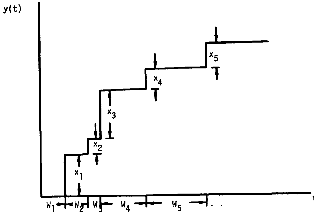
Fig 23. Hypothetical Distribution of Parts Failures, N(t) , as a Compound Poisson Process.
