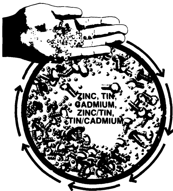
CROSS-SECTION OF BARREL TUMBLING FASTENERS
