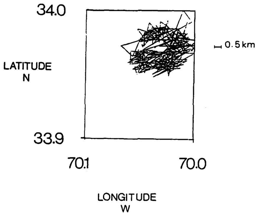
**Figure 12. Position of LOTUS-3 during June and July 1982 as tracked by the ARGOS satellites. The accuracy of the positions, 0.5 km, is shown as a scale. The dot marks the anchor position. The lines connect the buoy position between successive satellite passes.**
