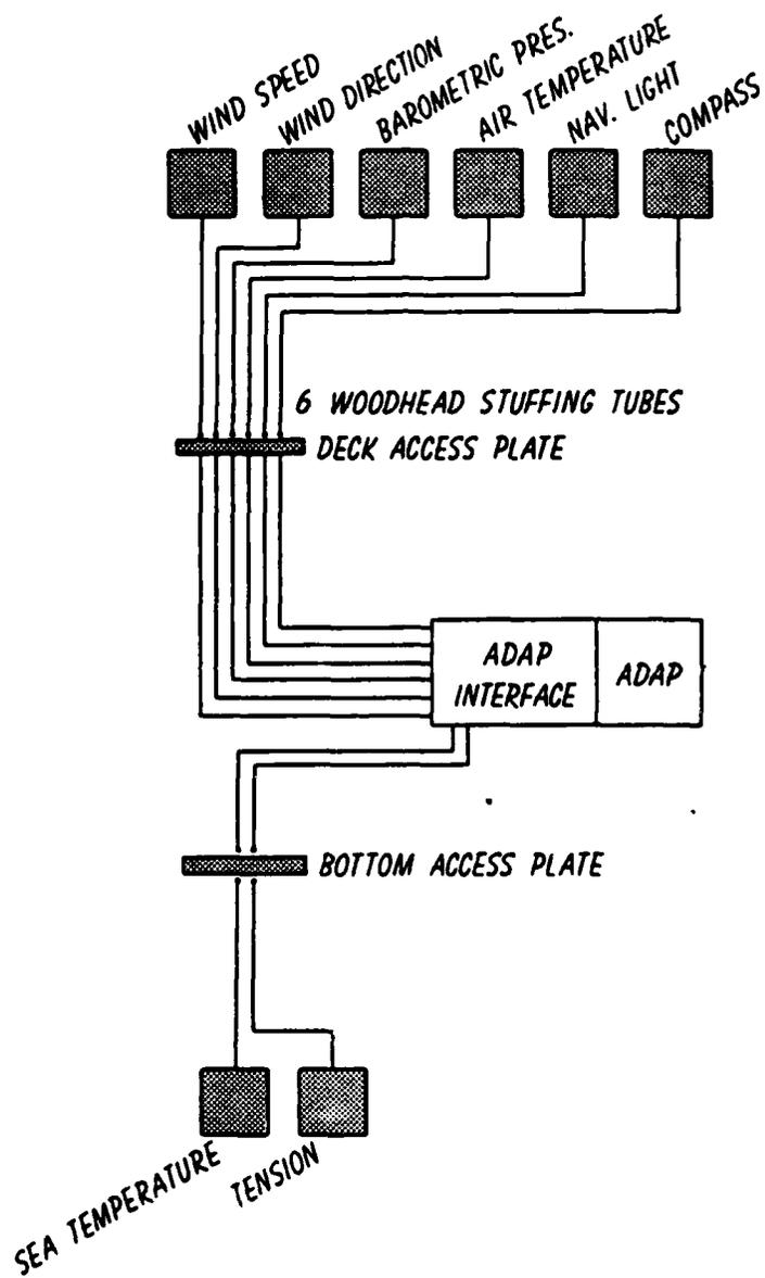
Figure 10. Schematic of the connections between the telemetered sensors and the ARGOS transmitter terminal (ADAP).
