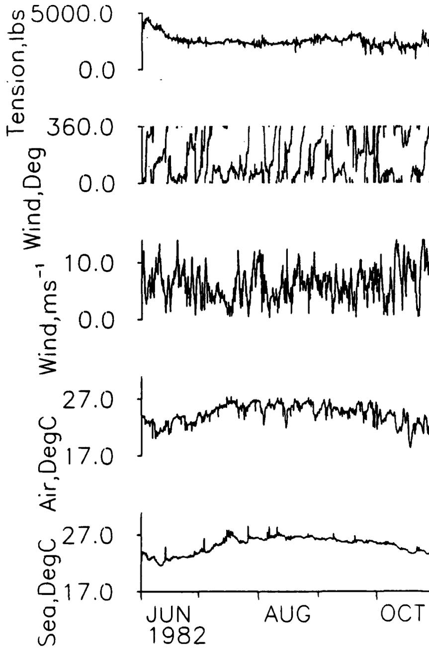
Figure 18. Time series of edited telemetered sea and air temperature, wind speed and direction, and tension along the mooring line.
