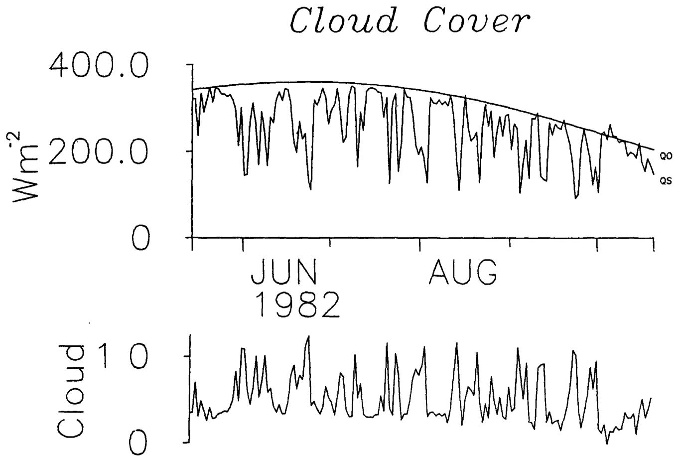
Figure 27. (a) Measured insolation (QS) augmented by  $60 W m^{-2}$ , and clear-sky insolation (Q0) in  $W m^{-2}$ . (b) Derived daily-averaged cloud cover in tenths, from LOTUS-3.
