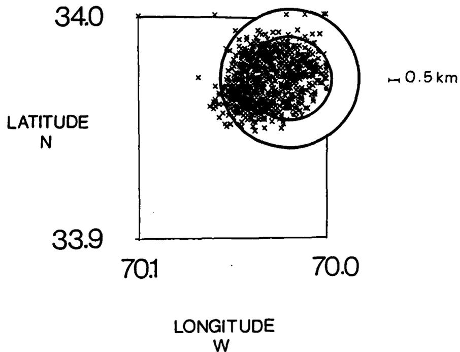
Figure 13. Position of LOTUS-3 during June to October 1982 as tracked by the ARGOS location system. The accuracy of the positions, 0.5 km, is shown as a scale. The watch circles (radii 3.45 km and 2.0 km) are centered at the anchor position. See text for explanation.
