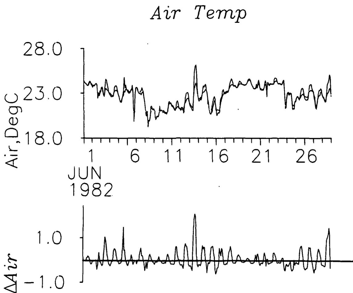
Figure 24. (a) Time series of air temperature from the Thaller- and PRL-shielded thermistors. The PRL housing overheats by 1°C-2°C during calm, sunny days. (b) Air temperature difference, during LOTUS-3.
