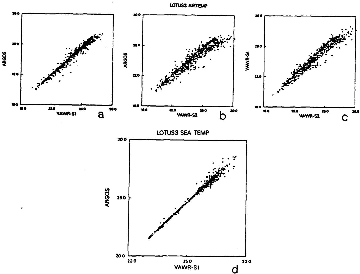
Figure 23. Scatterplots of two-hour averaged air and sea temperature from LOTUS-3. See Table 6 for the regression statistics.
