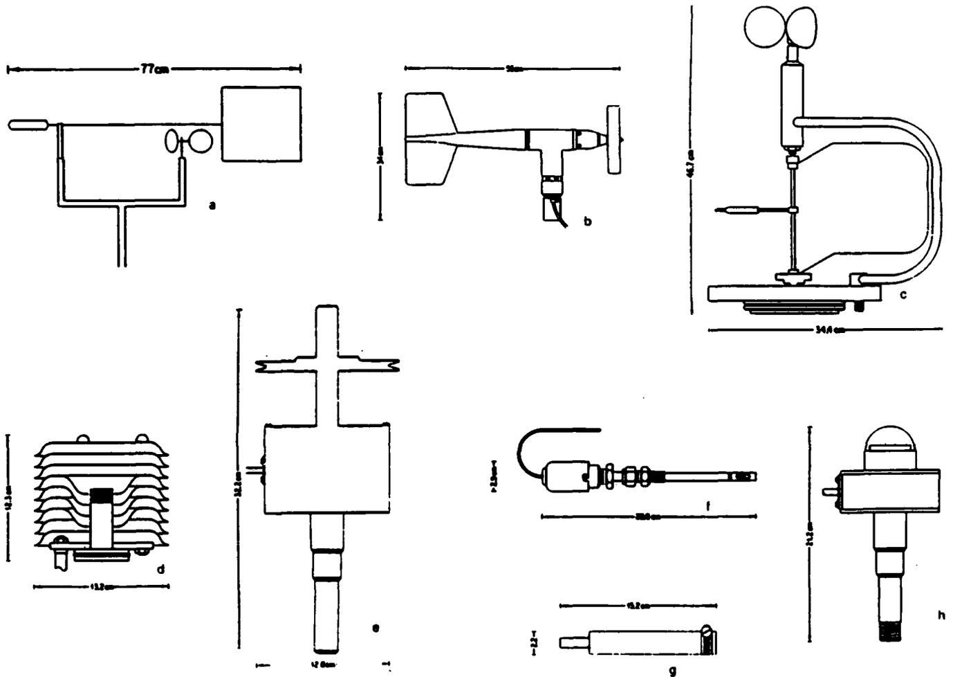
Figure 6. Schematic diagrams of the meteorological sensors on LOTUS-3 and LOTUS-4: (a) Gill 3-cup anemometer and vane, (b) Young 5101 Wind Monitor, (c) Integral 3-cup anemometer and vane, (d) Air temperature thermistor with Thaller shield, (e) Digiquartz barometric pressure case with pressure port (f) Bycal relative humidity sensor, (g) Sea temperature thermistor (h) Pyranometer.
