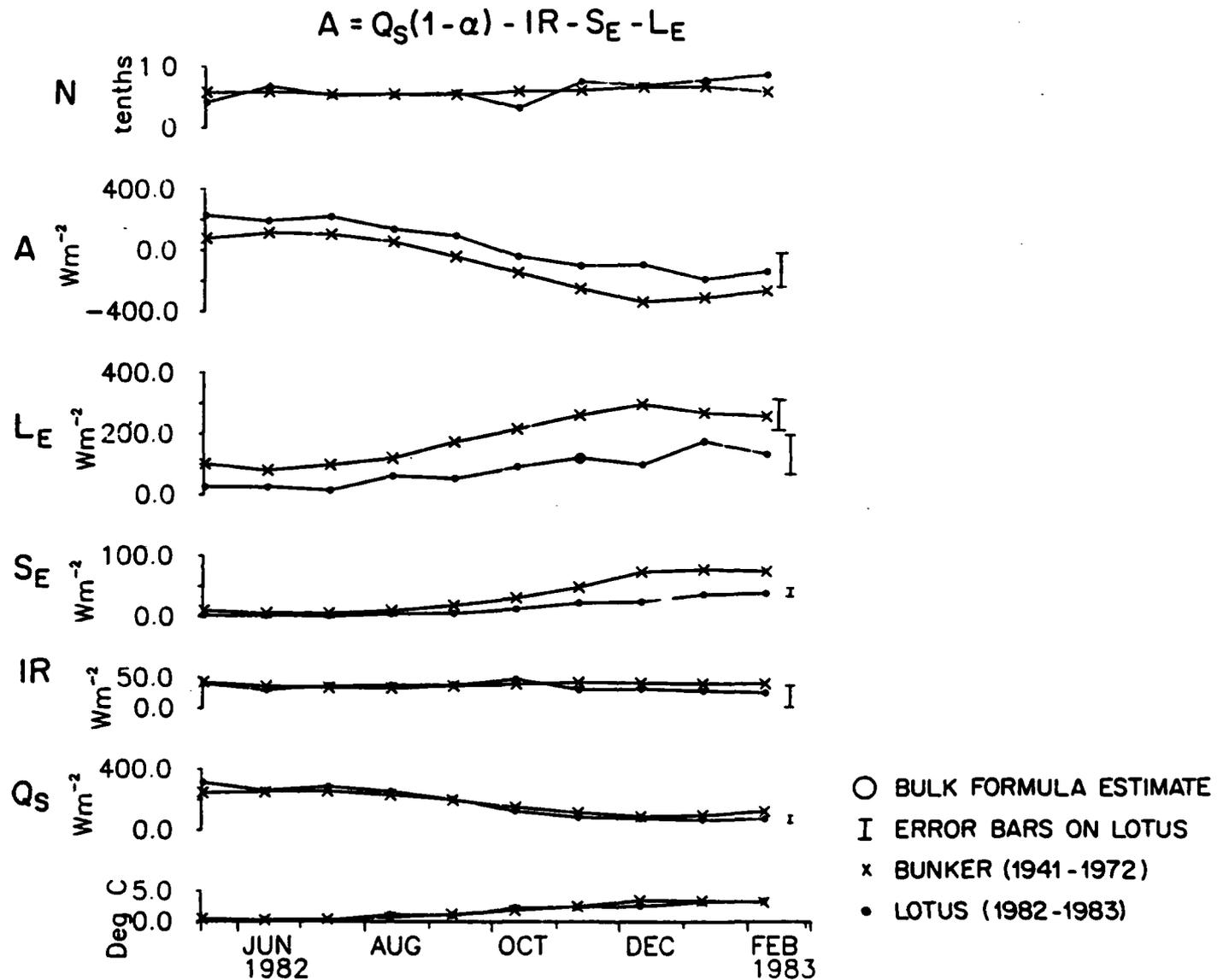
Figure 26. Comparison of heat fluxes from the monthly-averaged LOTUS data (•) and from Bunker's 32-year monthly means (x) (Bunker, 1975). From the top, N is cloud cover, A is net heat gain/loss by the ocean,  $L_E$  is latent heat flux,  $S_E$  is sensible heat flux, IR is net longwave radiation flux,  $Q_S$  is solar radiation, and sea minus air temperature.
