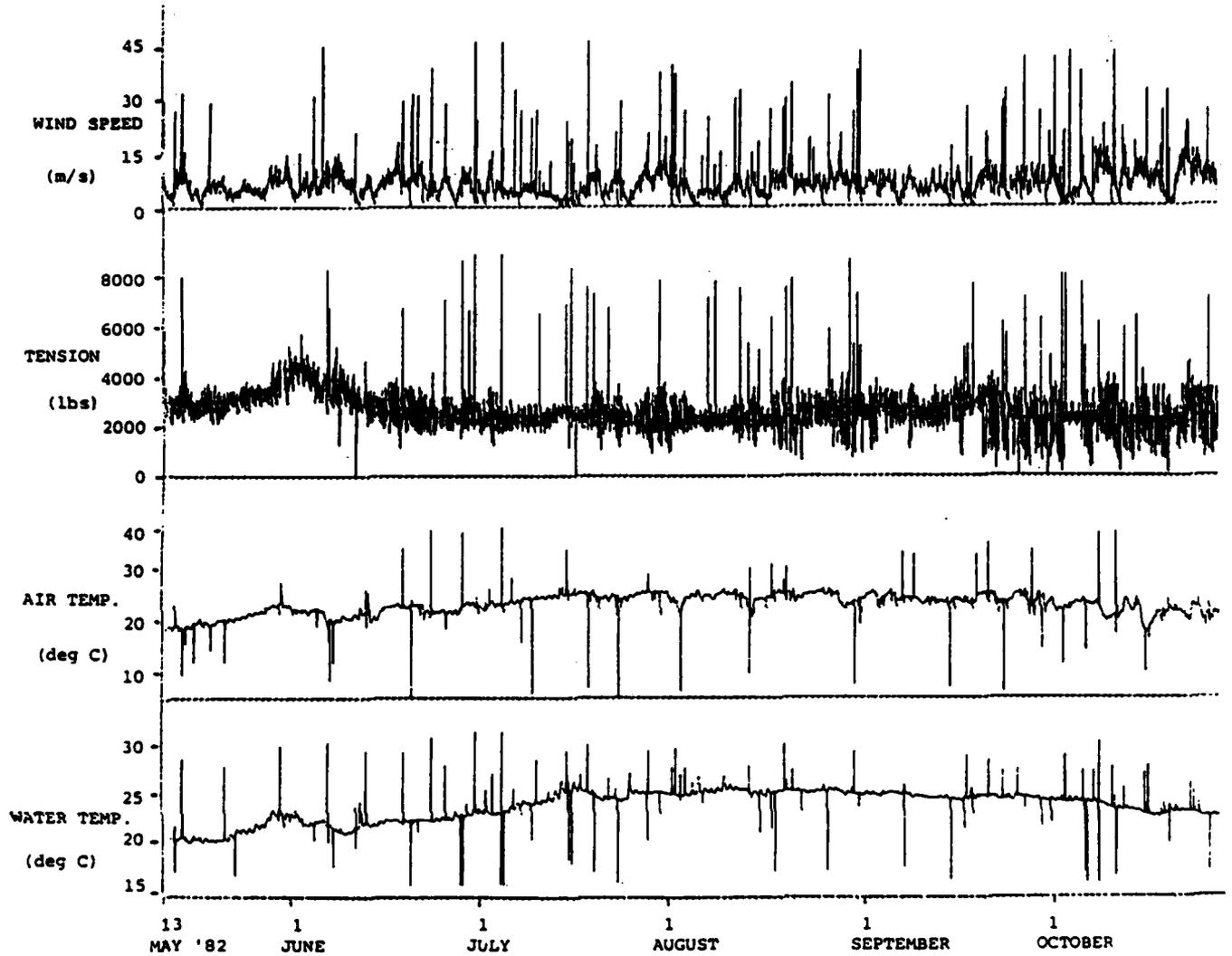
Figure 16. Unedited time series of telemetered sea and air temperature, tension along the mooring line, and wind speed.
