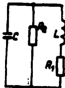
Fig. 65. The equivalent diagram of the parallel oscillatory circuit: C and L - capacity/capacitance and the inductance of duct/contour; R_1 - resistor/resistance of insertion losses and losses in the capacity/capacitance; R_2 - resistor/resistance of losses in the inductance.
