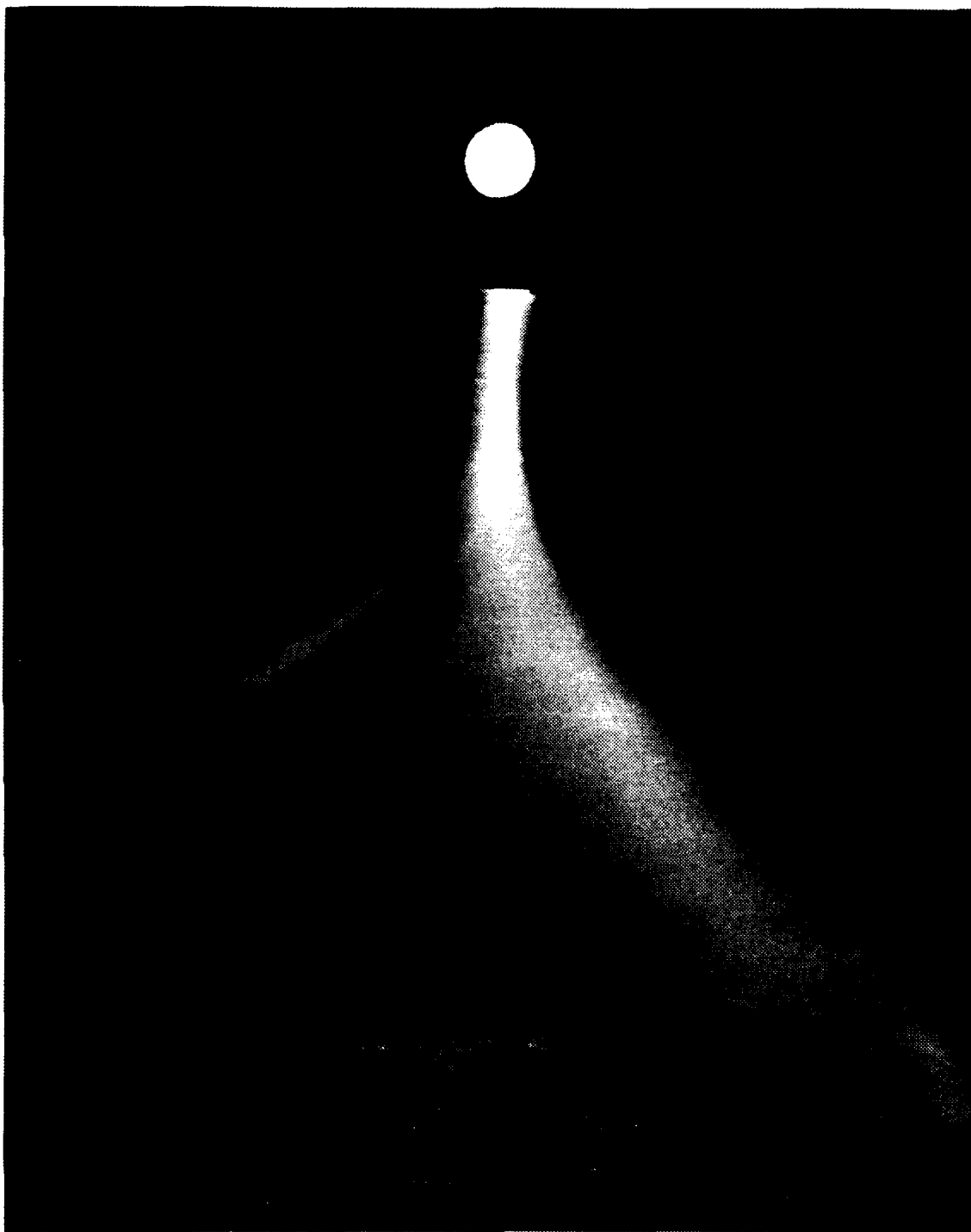
Figure 12. Open shutter photograph of the FX-25 beam extracted into full-density air (630 Torr) through a 25 m Kapton foil after drifting through 3 m of 3 Torr air.
