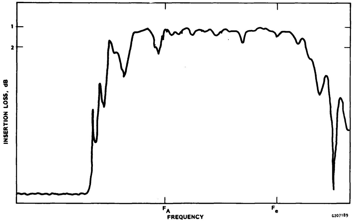
Figure 13. Anode Insertion Loss, Model No. 4, Sealín.
