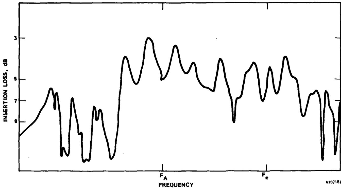
Figure 11. Cathode Insertion Loss Model No. 4, Coaxial/Waveguide Transitions on Cathode Input/Output.
