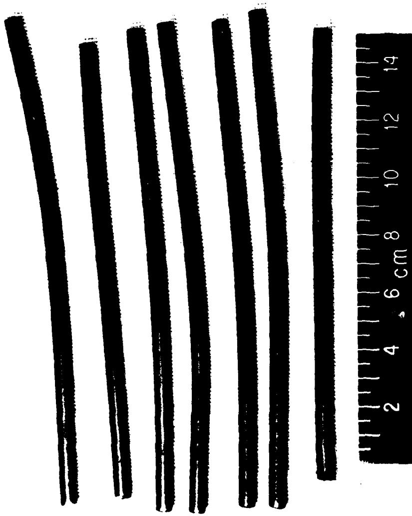
Figure 12. Extinguished Pieces of Short, Large-Perforation, Unslotted, NOSOL 363 Stick Propellant
