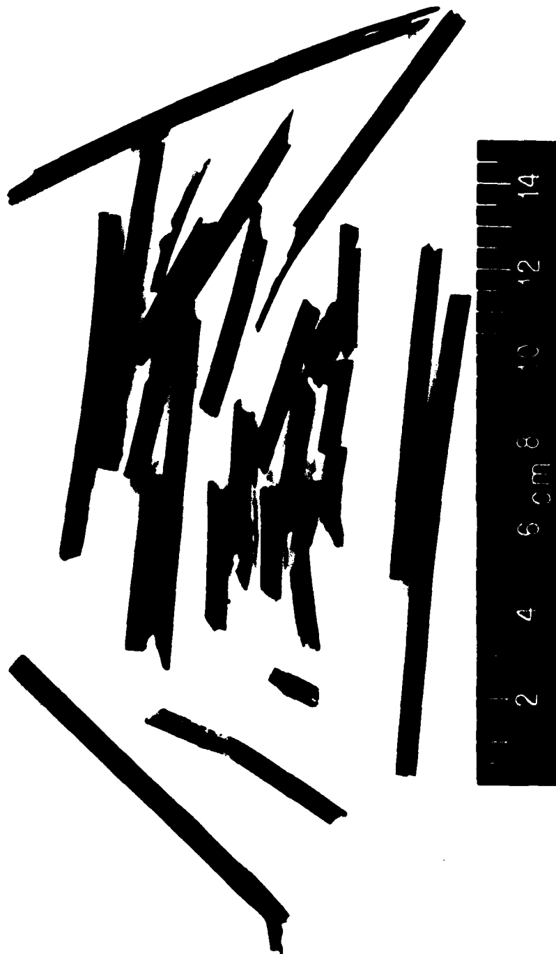
Figure 13. Extinguished Pieces of Long, Small-Perforation, Unslotted, NOSOL 363 Stick Propellant
