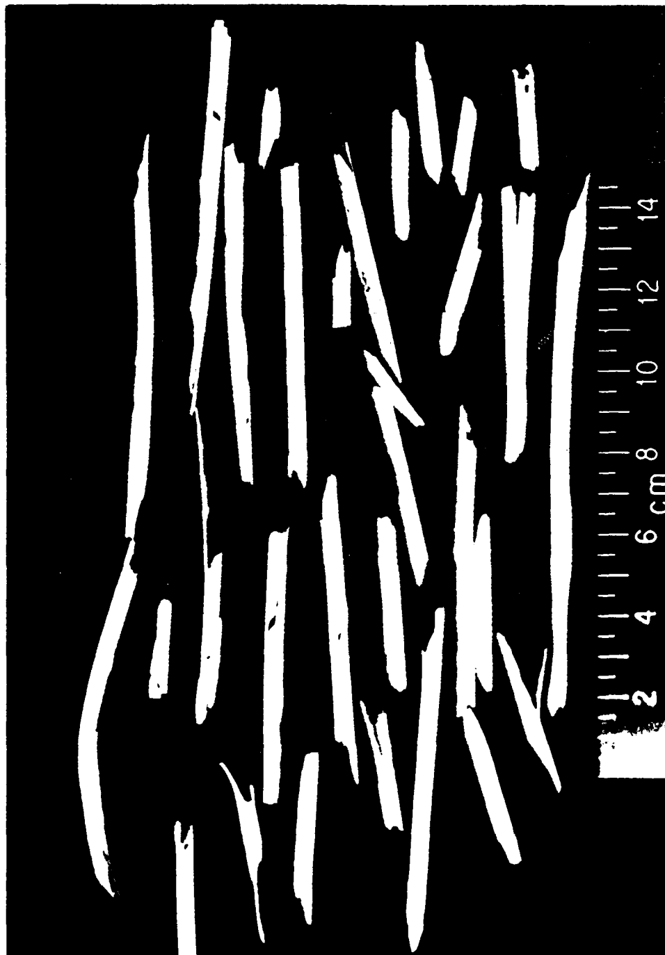
Figure 15. Extinguished Pieces of Long, Slotted, M30A1 Stick Propellant, Lot RAD 472-11
