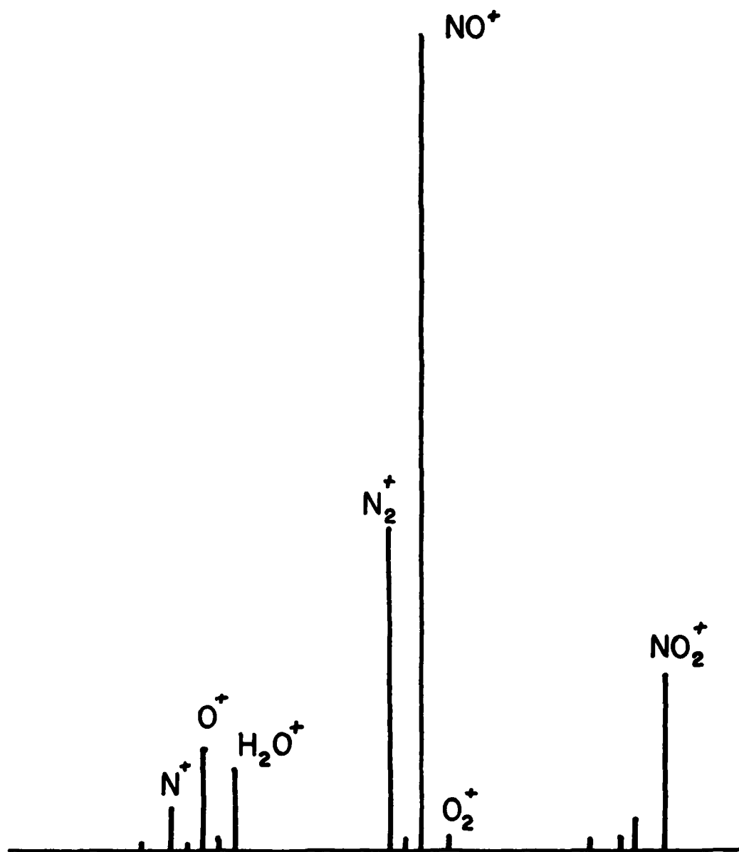
Fig. 1 Mass Spectrum of \text{NO}_2 and \text{N}_2\text{O}_4 ( -30^\circ\text{C} )
