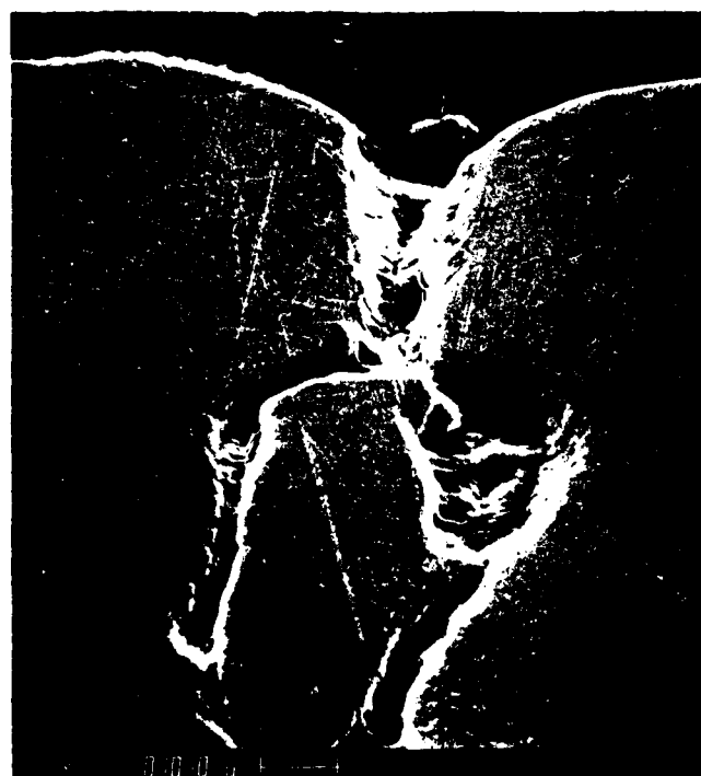
Figure 32 SAME CRACK AS ABOVE AT 1000X. PROPELLANT GASES HAVE ERODED CRACK WIDTH TO 10-15 \mu = 0.5 MIL
