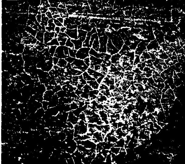
SURFACE OF HARD CHROME PLATED EROSION SENSOR AFTER ONE SHOT (100X, SEM)
