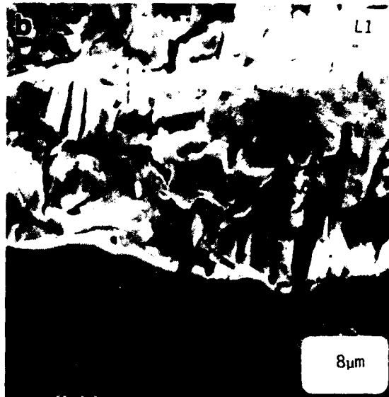
Fig. 13 - Precision sectioning SEM micrographs for (a) hypotransitional, and (b) hypertransitional FCGR behavior for condition L1
