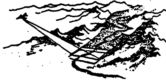
Figure 4. An airplane equipped with a CCD camera doing inclination photography
