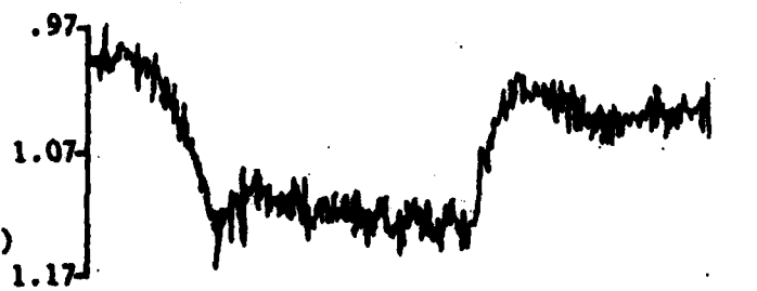
Figure 6.3 Example of seat sensor array output during 30°, 6°/sec coordinated turn
